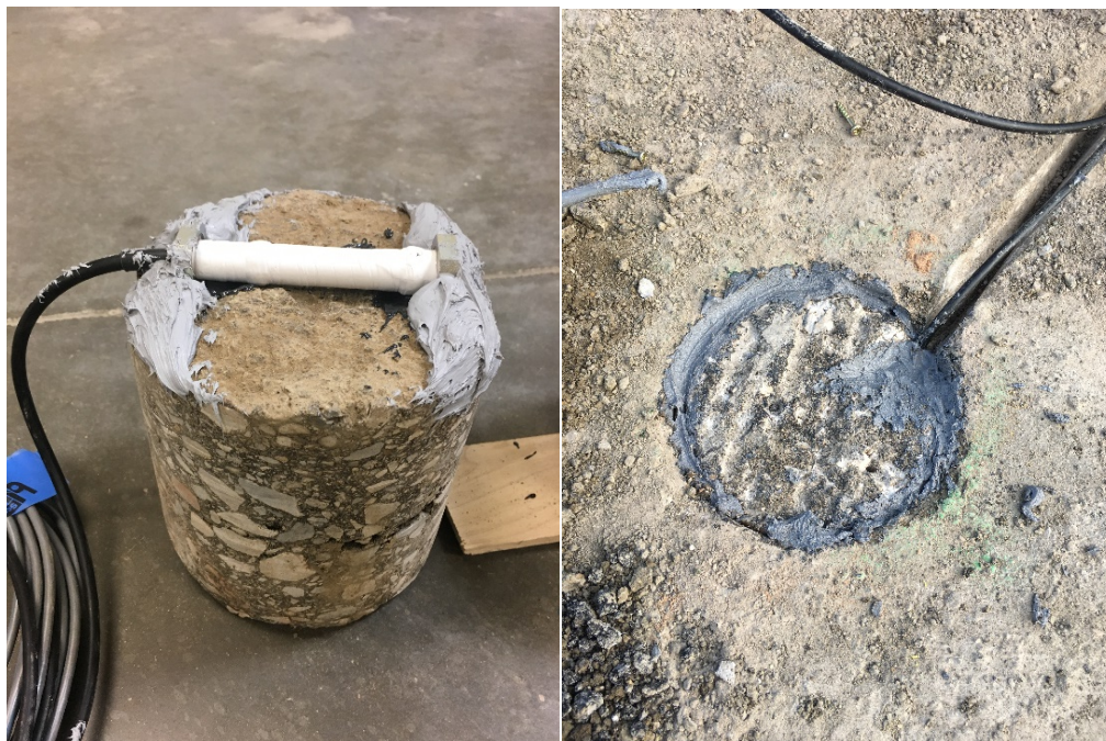
Figure 27. Strain gauge glued to the HMA Core.
