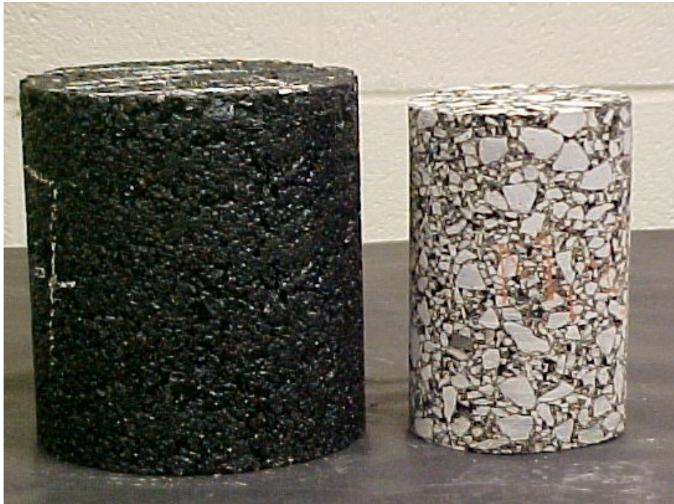
Figure 17. Sample obtained from Superpave Gyrotory Compactor (SGC).
