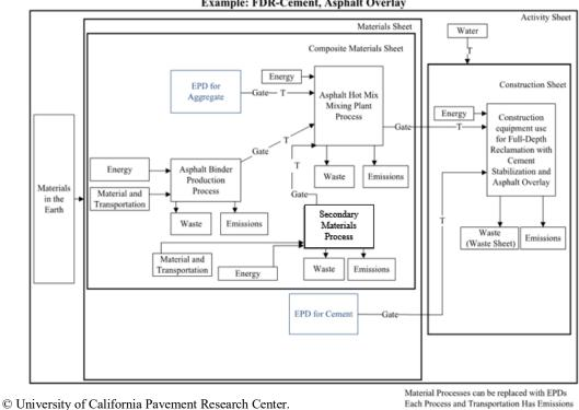
Activity Sheet, Materials Sheet, Composite Material Sheet, Construction Sheet Example: FDR-Cement, Asphalt Overlay
