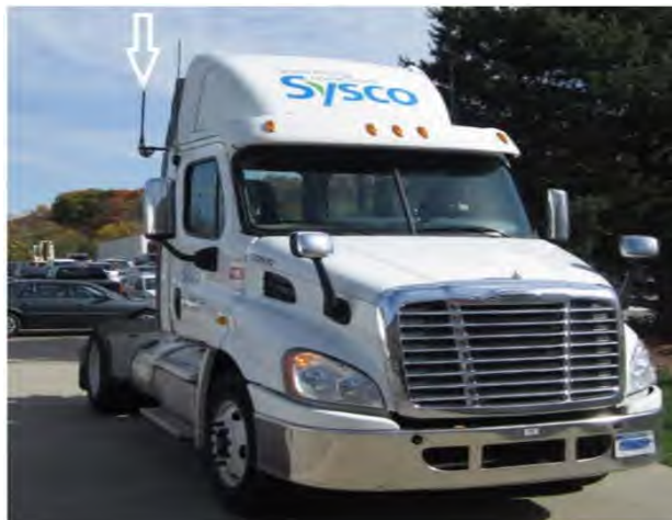
Figure 51 A truck equipped with the RSD device and DSRC antennas (pointed by an arrow).
