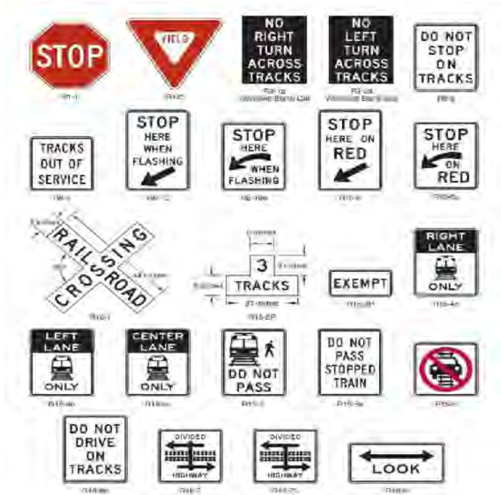
Figure 32 Regulatory signs and plaques for highway-rail grade crossings. Source: MUTCD. (2009). Manual on Uniform Traffic Control Devices (Figure 8B-1)
