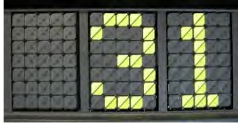
Figure 42 An example of a flip disk or flip dot display. Source: Wikimedia Commons. (2020). Flip-dots
