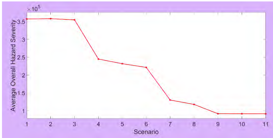
Figure 135 The average overall hazard severity over all the PF points for each countermeasure availability scenario.
