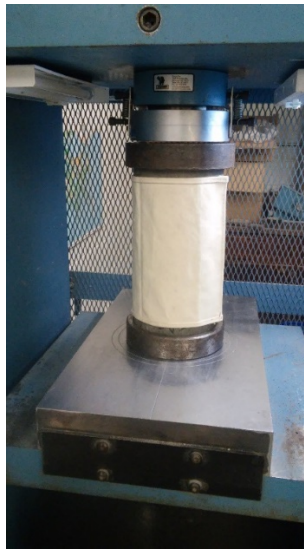
Figure 4. Compressive strength test setup.
