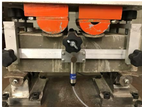
Figure 6. Third-point bending test setup.
