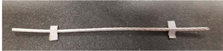
Figure 10. Sample braided wire before testing with a gauge section of 50 mm. Two rectangular attachments represent laser tags for strain measurement.
