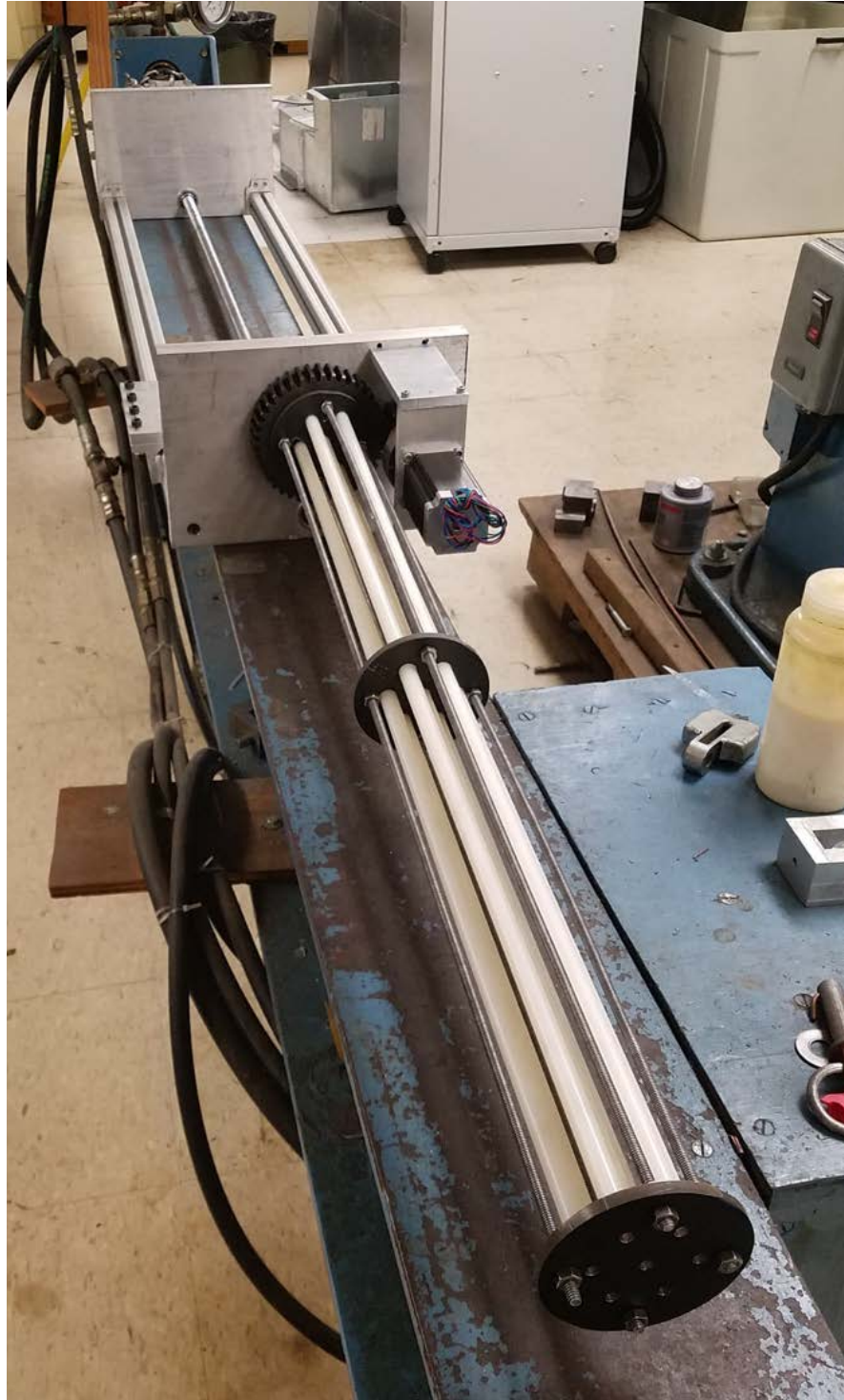
Figure 23. Finished experimental setup for fabricating braided cables.
