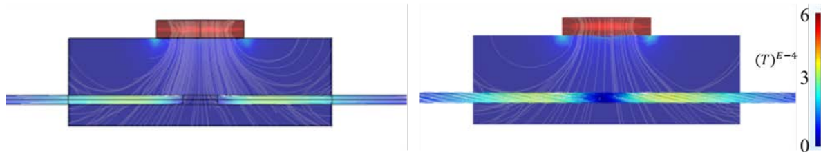
Figure 16. A large wire (left) and braided cable (right) of the same cross-sectional area are created to compare a cable configuration. The cable consists of 6 wires braided around a straight wire of the same size. While the single wire has a consistent magnetic flux across the cross-section, the braided cable shows a more consistent flux along the individual wires.
