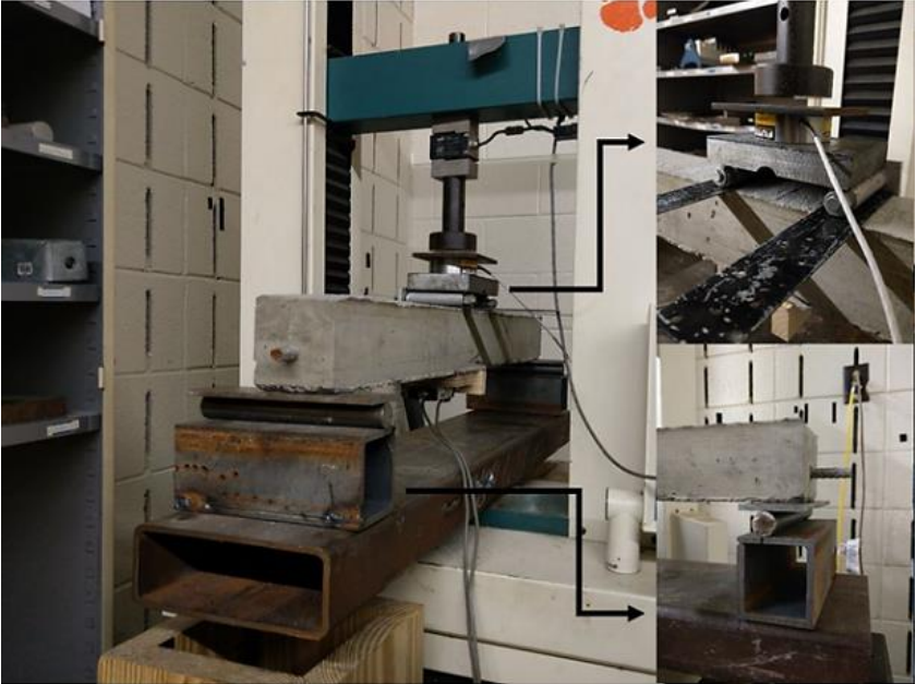
Figure 24 - Short beam test set-up.
