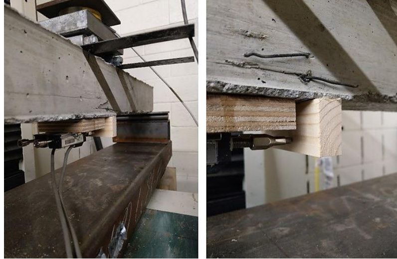
Figure 25 - Linear potentiometer set-up using woodblocks.
