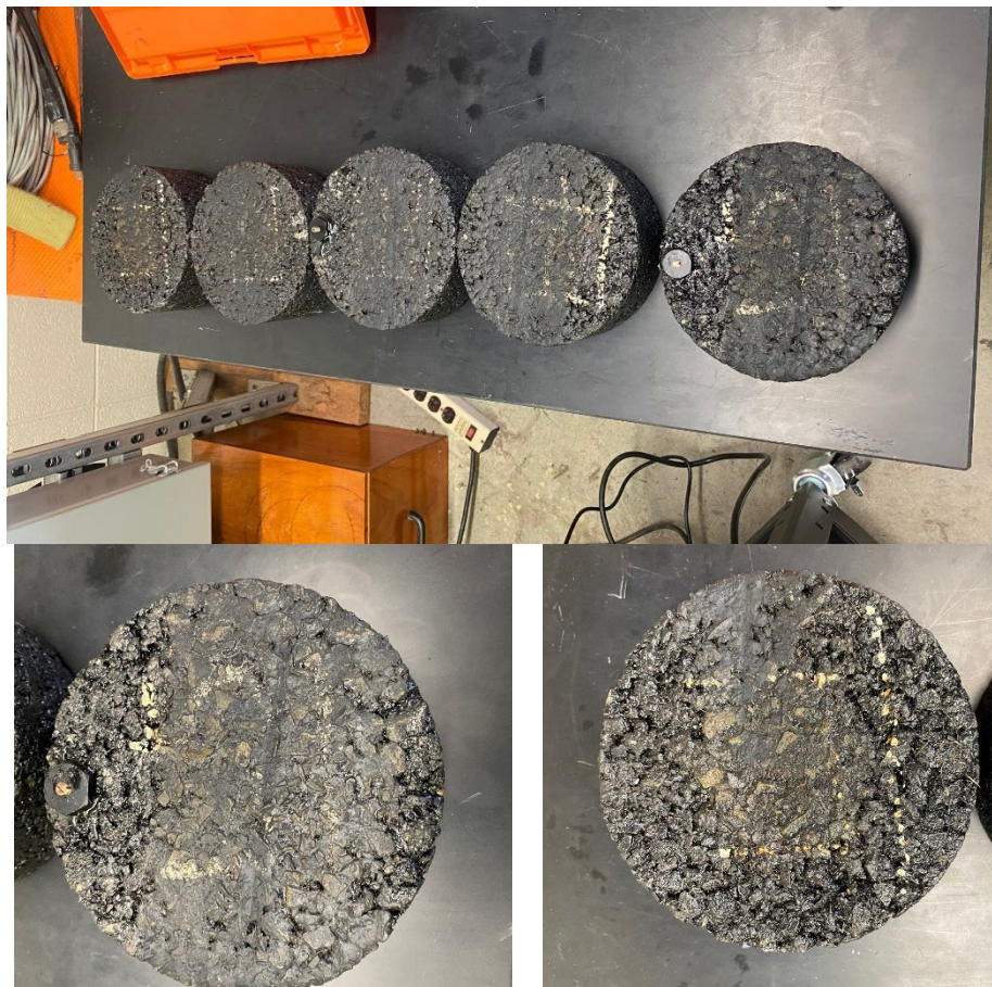
Figure 26. The specimens after the MMLS3 test
