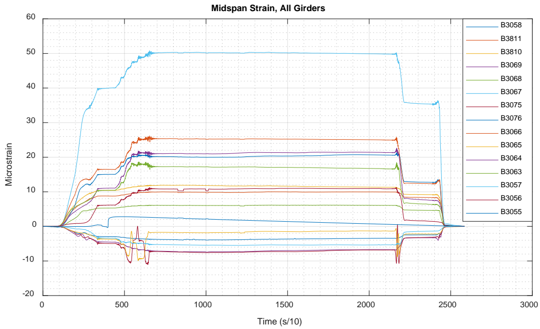
Figure 21: Bridge 5489 SBS_S_2_1 strains - Midspan
