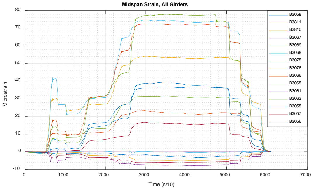
Figure 97: Bridge 3848 MAX_S_2_1 strains - Midspan
