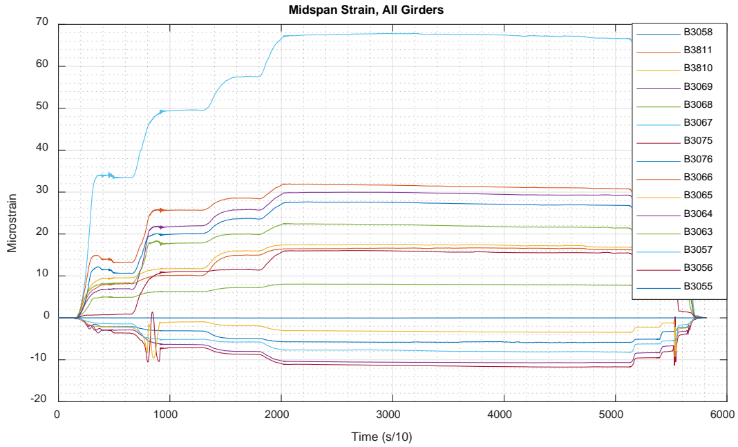
Figure 29: Bridge 5489 ALT_S_2_1 strains – Midspan
