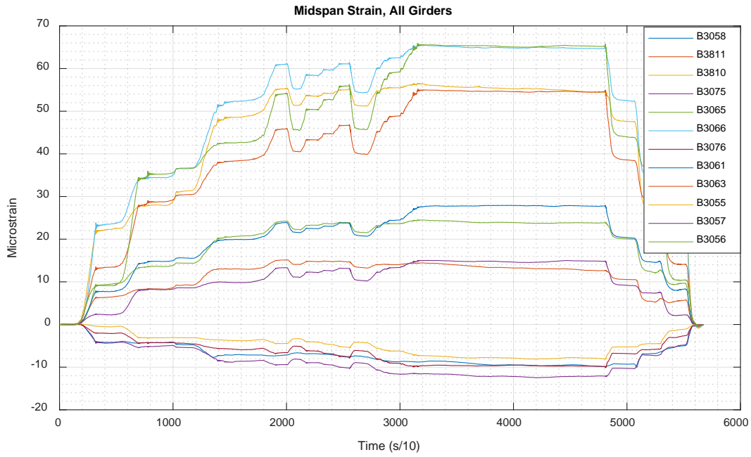
Figure 79: Bridge 2879 MAX_S_2_1 strains - Midspan
