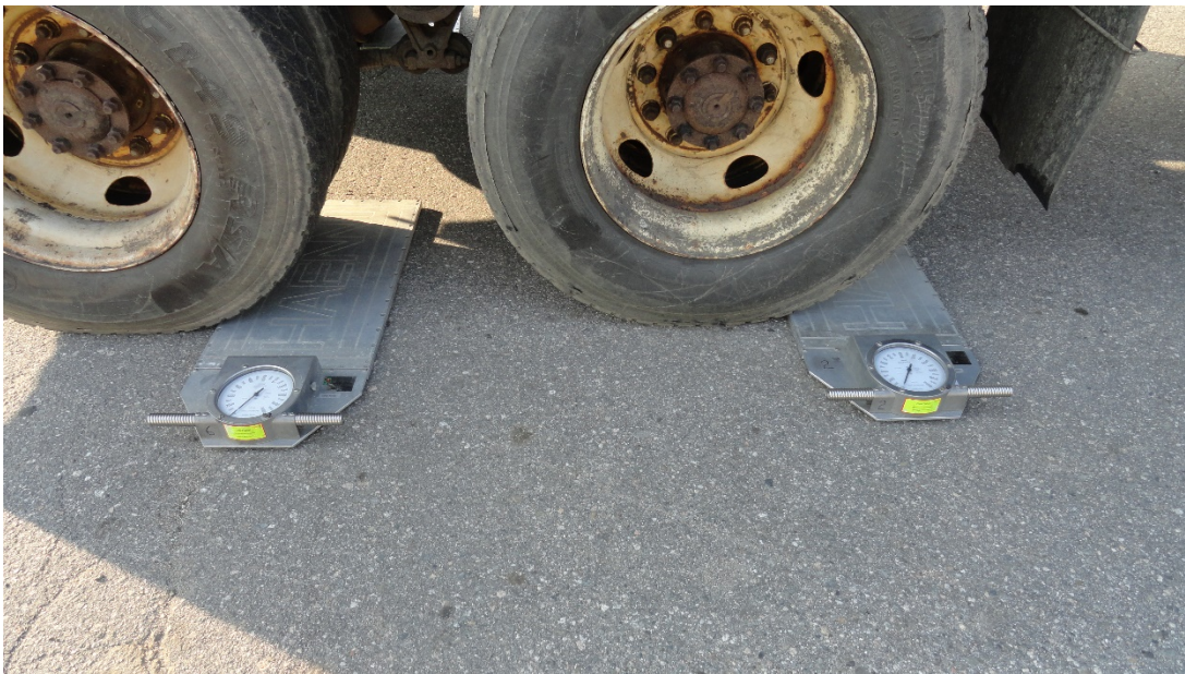
Figure 5: State highway patrol certified portable truck scales used to verify vehicle weight for each test
