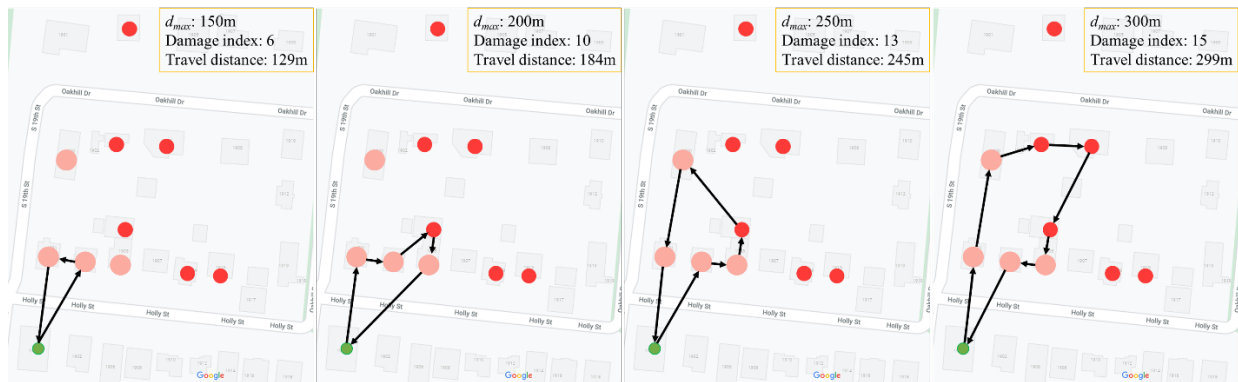
Figure 4-8 Optimized UAV Mission Plans for Different Distance Constraints.
