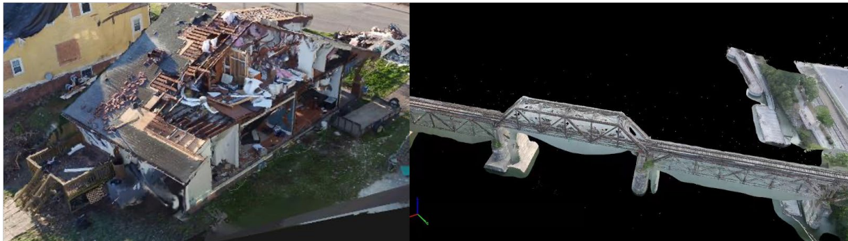
Figure 3-1 3D Reconstruction of Structures from Drone-Collected Images.
