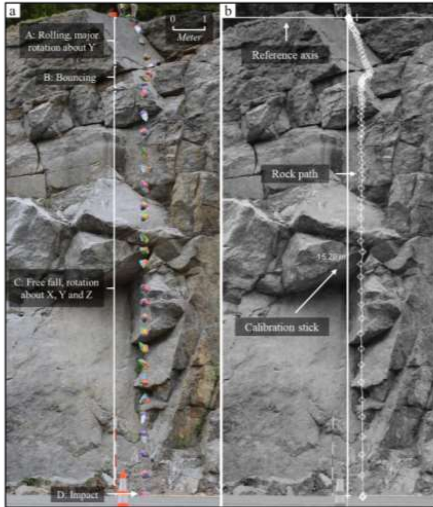
Figure 5. Rockfall trajectory for rock 6, Warner, NH: (a) combination of video frames, and (b) tracker software. The calibration of each video analysis was based on the known drop heights, measured with a total station.
