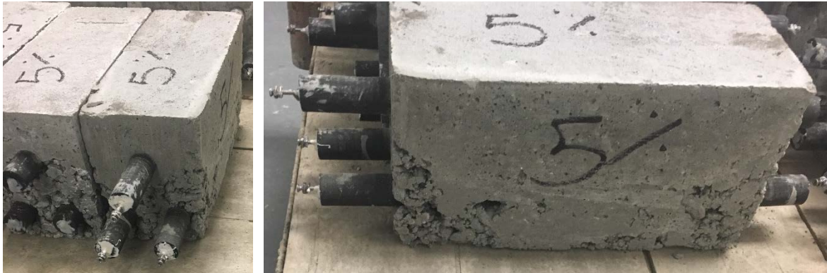
Figure 19. Honeycombing observed in TEA-C 5.0% specimens.
