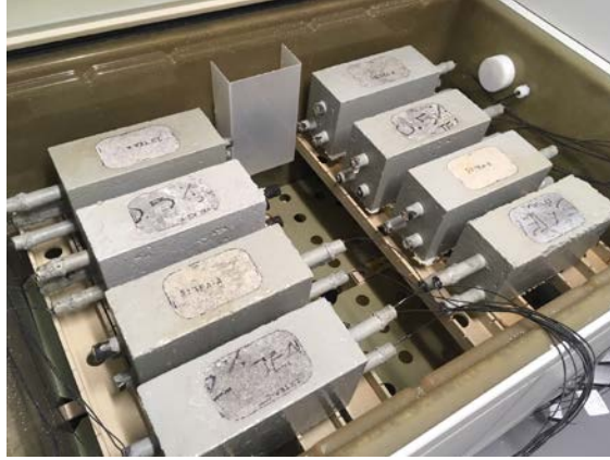
Figure 11. Three electrode system set-up for the fog chamber samples.
