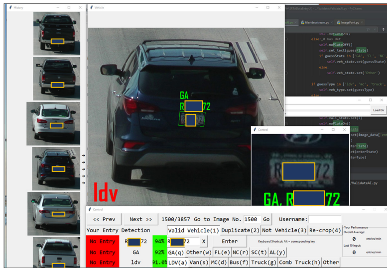
Figure 142 – Manual Verification User Interface
