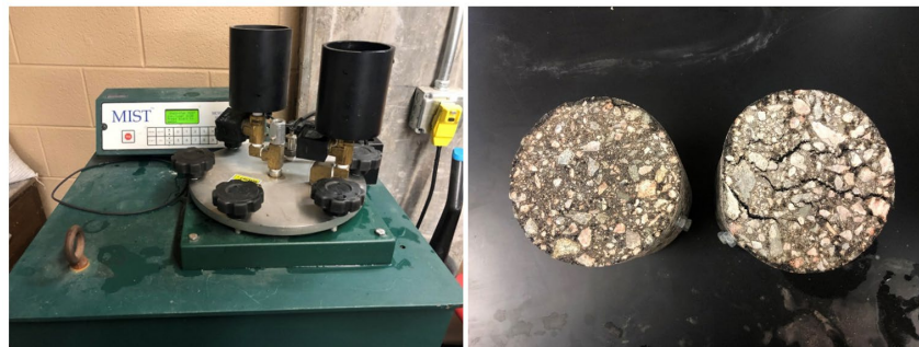
Figure 4-19. The AMPT samples before and after MIST conditioning at 60 °C
