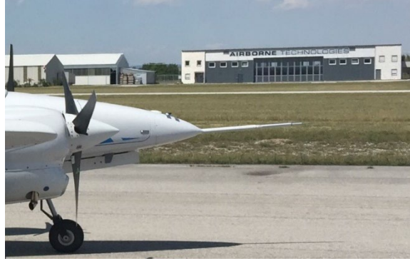
Figure 18. Five-hole Smart Air Data AOA source
