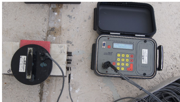
Figure 3. In situ i_{corr} measurement using a ring probe.
