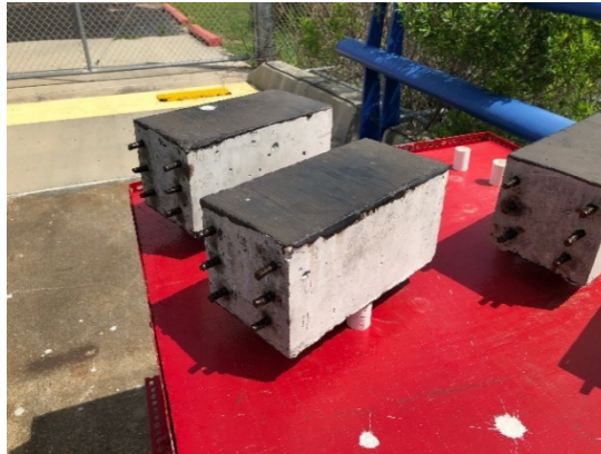
Figure 4. Concrete prism samples in the seacoast exposure in Galveston.
