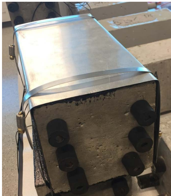
Figure 5. Concrete prism sample covered by the aluminum electrode.
