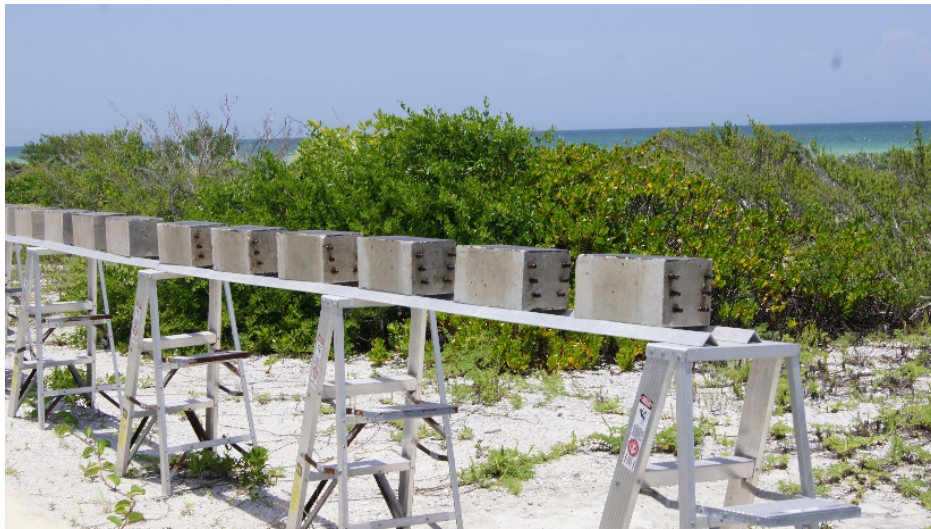
Figure 2. Concrete samples in the seacoast exposure in Mexico.
