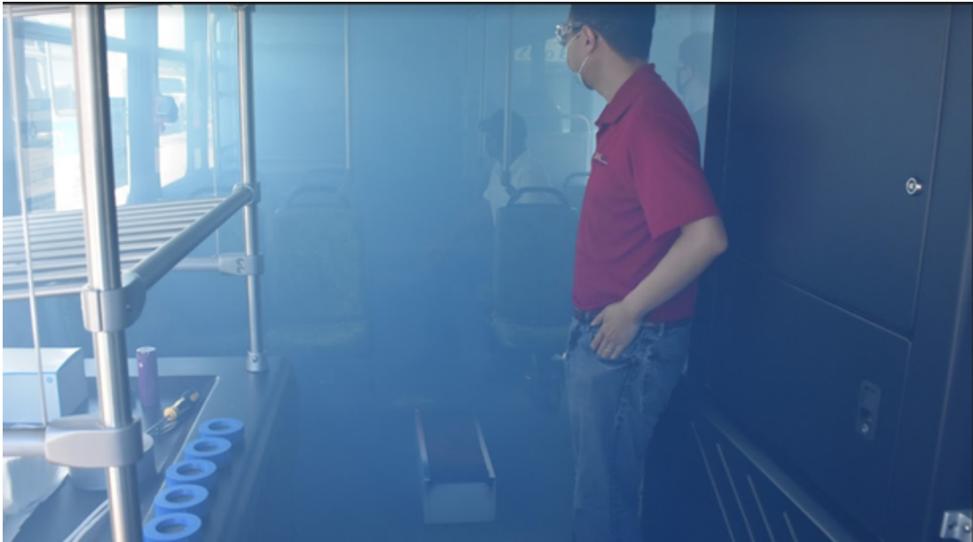
Figure 4: Interior Bus B, Smoke Testing
