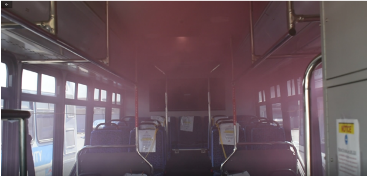
Figure 9. Experimental Smoke Visualization of the Interior Stationary Bus A Viewing from the Front
