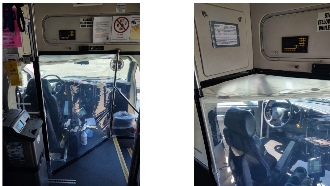
Figure 19: Two Photos Depicting the City of Clovis Transit's Flexible Plastic Enclosure to Protect the Drivers
