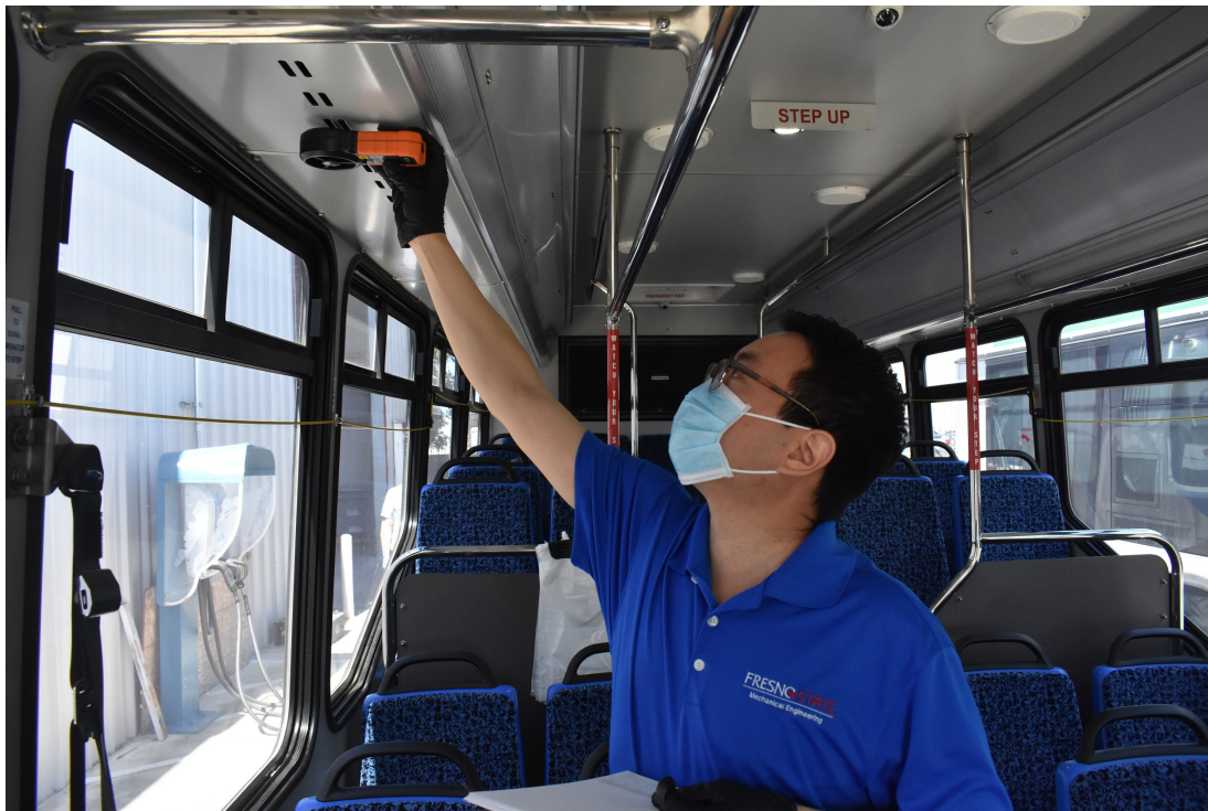
Figure 2. Airspeed from HVAC Ducting being Measured
