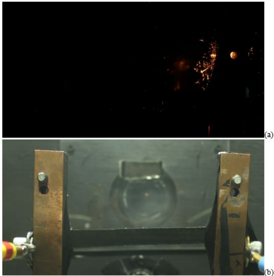
Figure 39. (a) Sample test image of contact sparking at the clamp area and (b) corresponding illuminated test setup for location reference.
