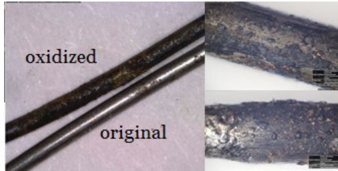
Figure 10. Comparison of new wire and wire that oxidized due to heating
