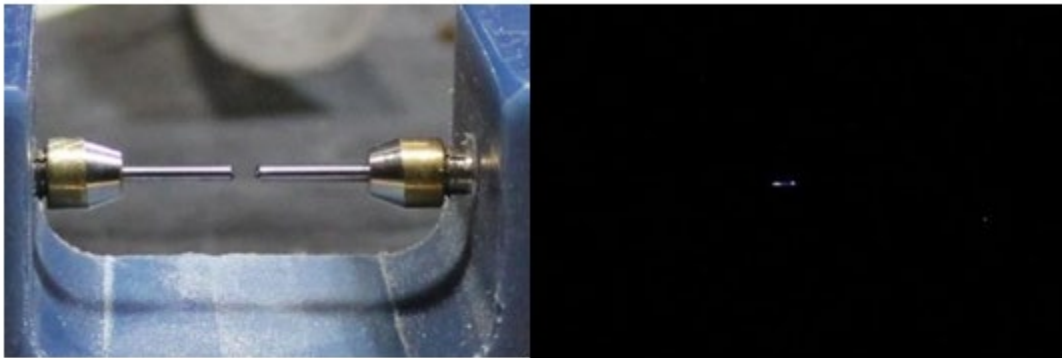
Figure 17. Voltage spark source used for White Paper calibration testing.
