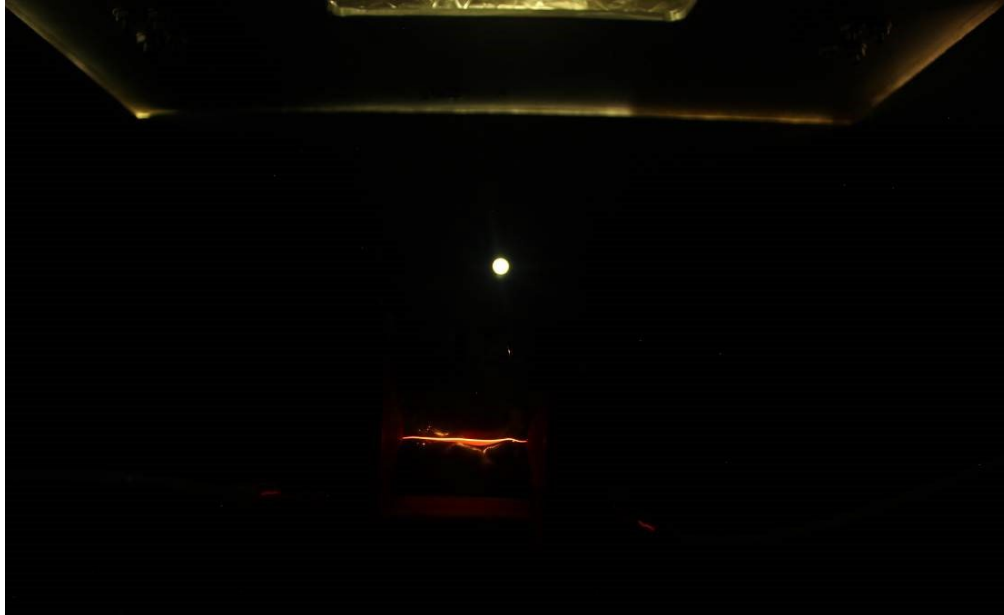
Figure 33. Sample photo of external light leaking into the test chamber.
