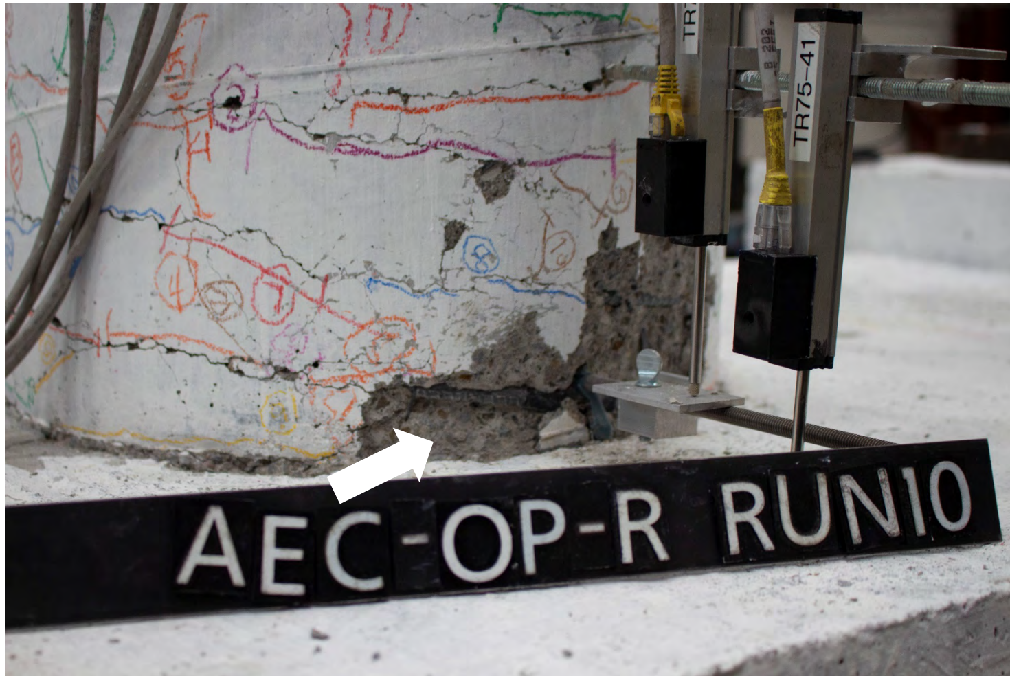
Figure 3.13 Concrete spalling in the north direction (run #10)
