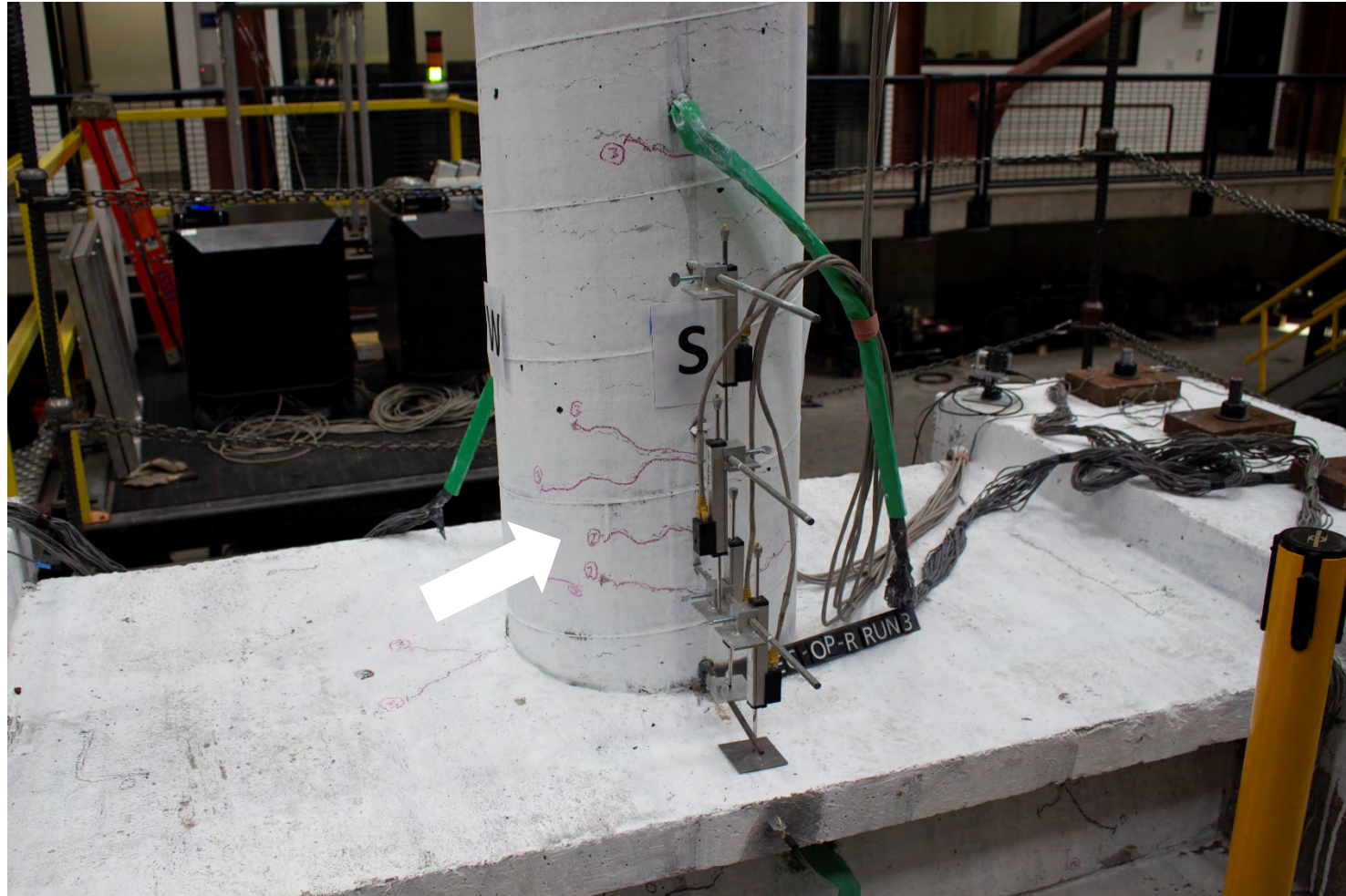
Figure 3.2 Additional flexural cracks (run #3)
