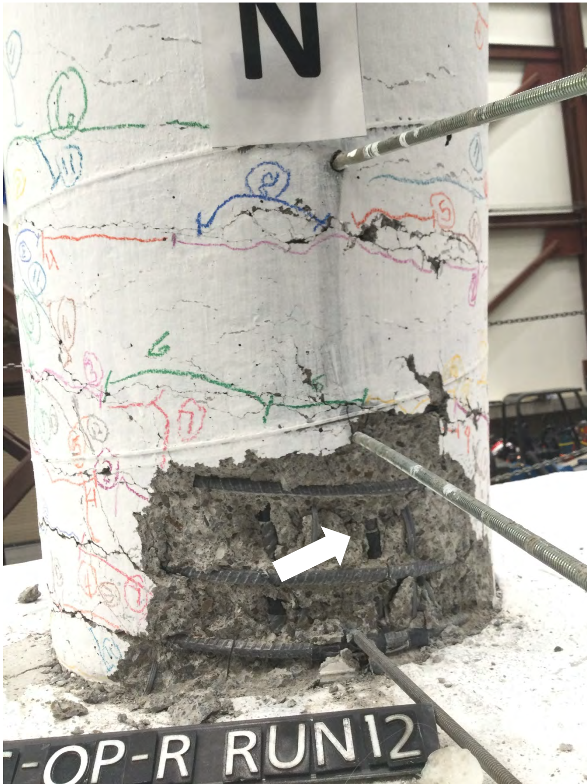
Figure 3.16 Spalling on the north side (run #12)
