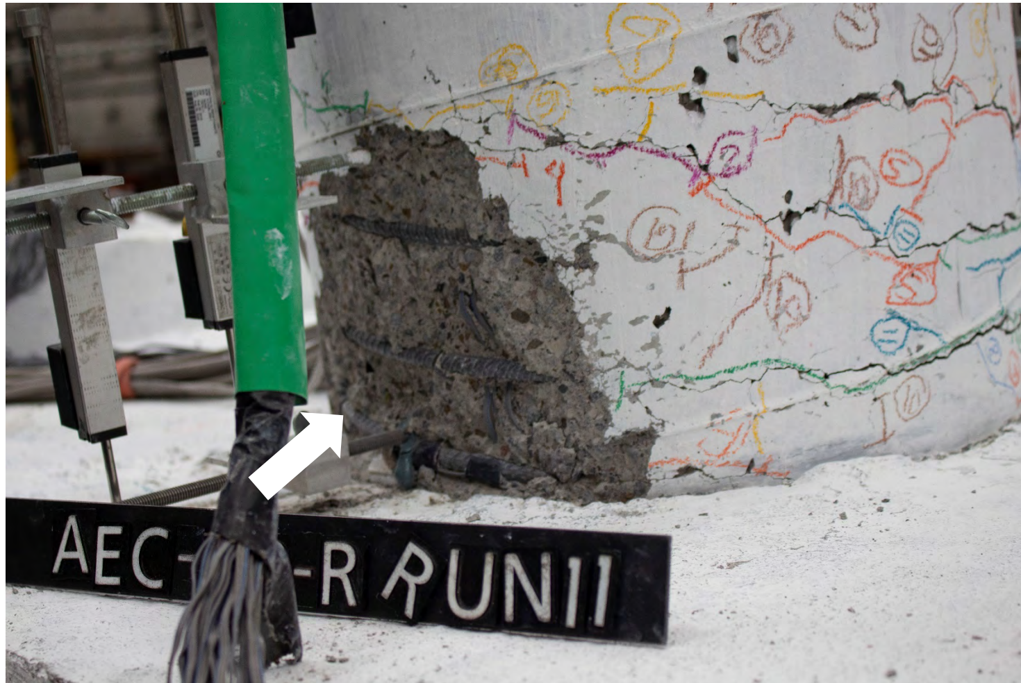
Figure 3.14 Concrete spalling in the north direction (run #11)
