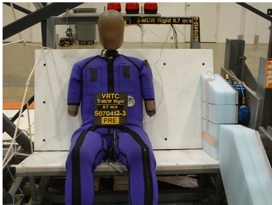
Figure 4-3. NHTSA 6.7 m/s padded flat wall test
