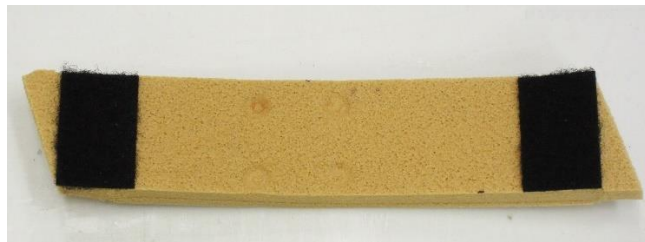
Figure 3-11. Velcro strips attach the individual pads to the corresponding ribs
