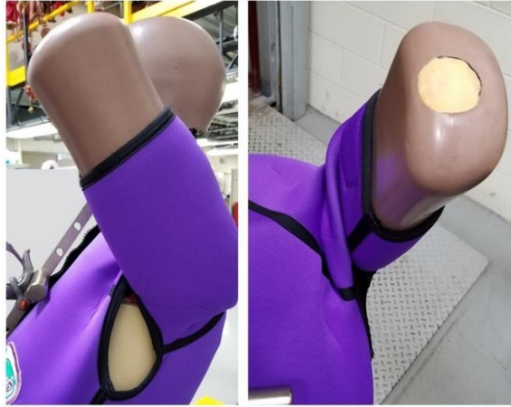
Figure 3-12. Sleeved Suit - hole under arm (left) and fabric bunching during shoulder flexion (right)
