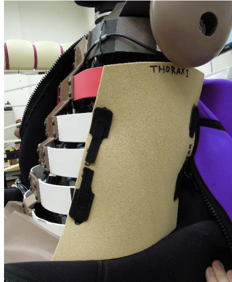
Figure 3-8. Original One-Piece Thorax Pad
