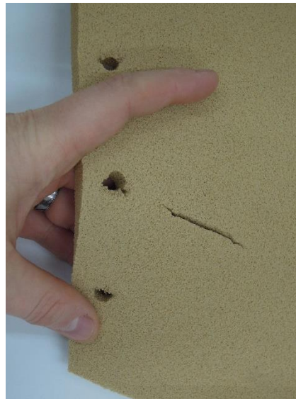
Figure 3-9. Typical Damage Observed in One-Piece Thorax Pad
