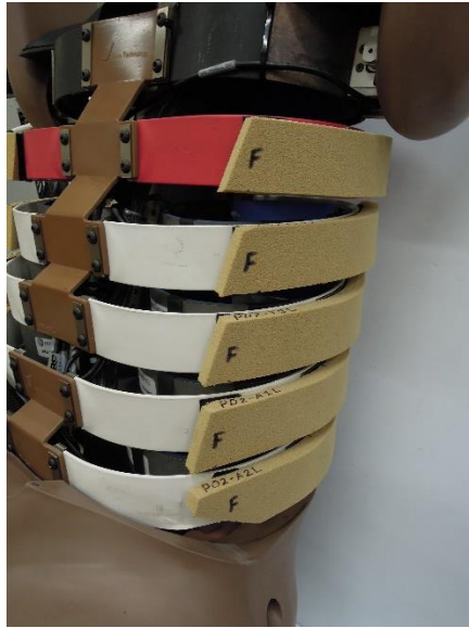
Figure 3-10. Split Thorax Pad Configuration
