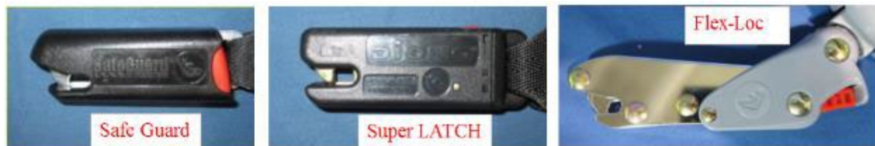
Figure 15. CRS Attachments Evaluated With Removable Lower Anchor Design
