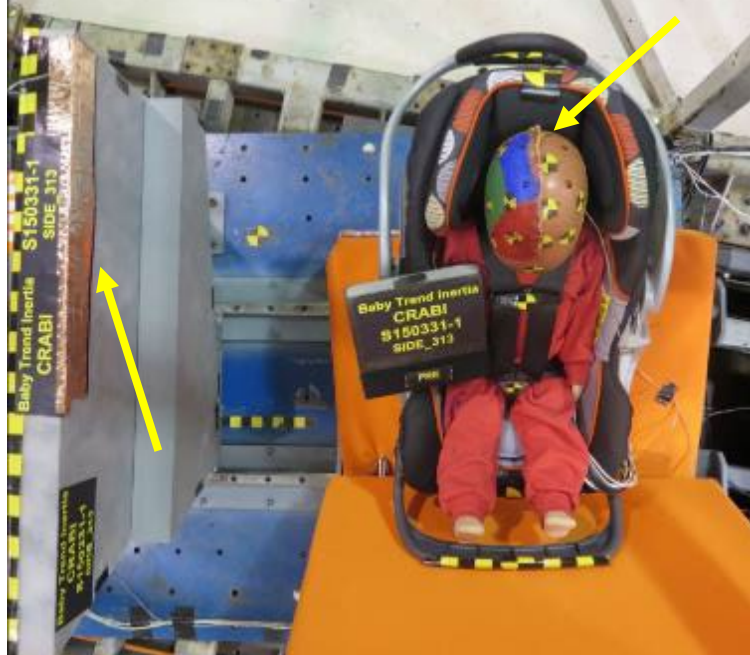
Figure D-9. Contact Tape and Copper Wire Mesh Example
