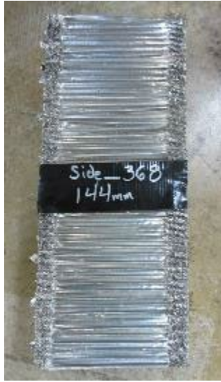
Figure D-26. Post-Test Honeycomb
