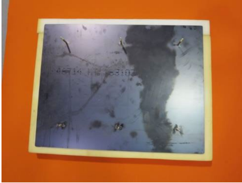
Figure E-2. Foam Placed on Plate With 25 mm of Foam on Each Side
