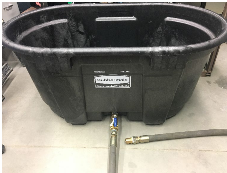
Figure 8. 100 Gallon Supply Tank and System Connection Hose
