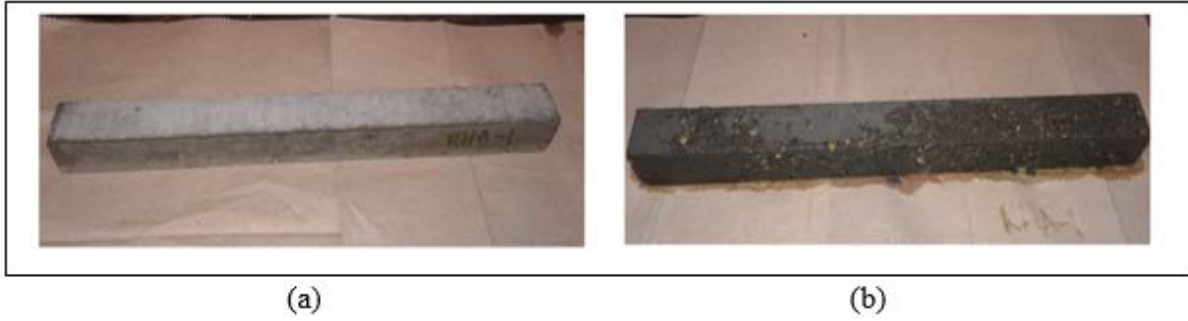
Figure 28. RHA-1-modified bar (a) before freezing and thawing cycle, and (b) after 10th freezing and thawing cycle.
