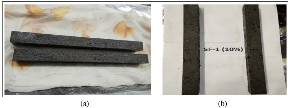
Figure 32. SF-modified bar (a) before freezing and thawing cycle, (b) after 10th freezing and thawing cycle.
