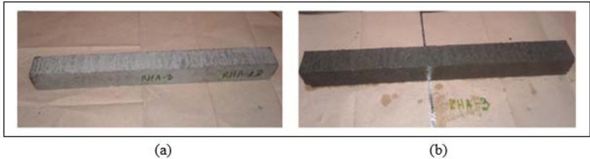
Figure 30. RHA-3-modified bar (a) before freezing and thawing cycle, and (b) After 10th freezing and thawing cycle.
