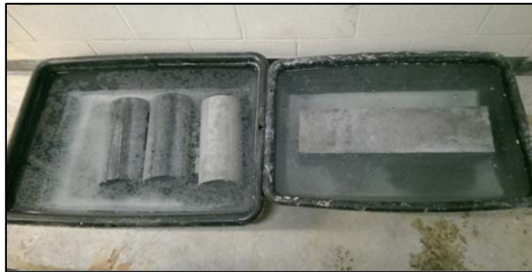
Figure 5. Curing process of concrete cylinder and beam samples.
