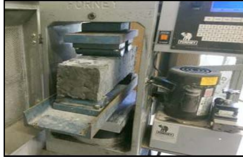
Figure 8. Flexural strength test with two-point loading set up.
