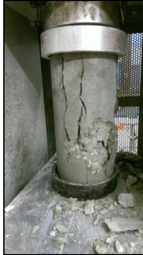
Figure 6. Compressive strength test.
