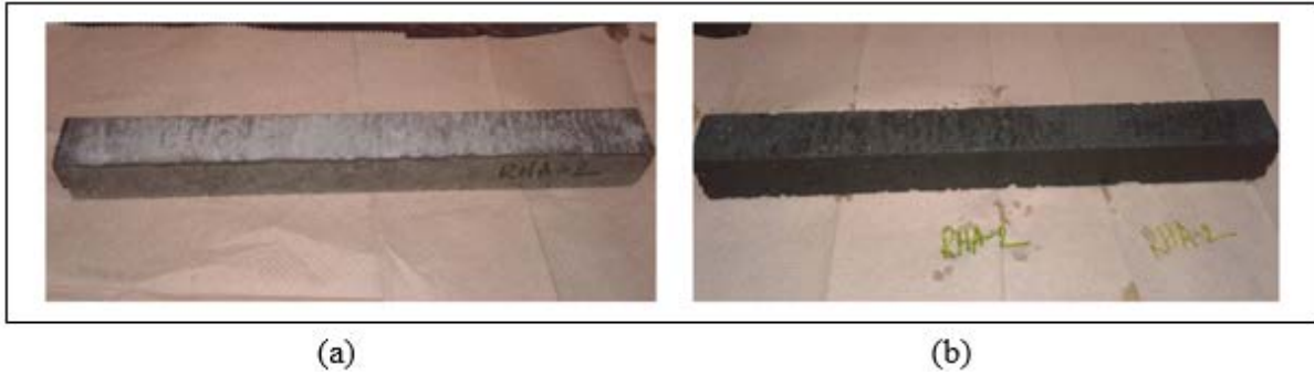
Figure 29. RHA-2-modified bar (a) before freezing and thawing cycle, and (b) after 10th freezing and thawing cycle.
