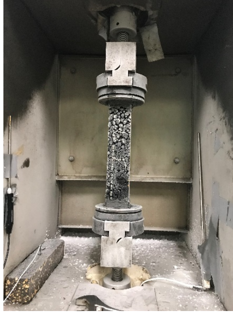
Figure 12. Thermal-stress restrained specimen test (TSRST).
