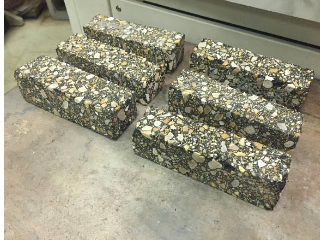
Figure 6. Rectangular beams prepared for crack healing efficiency.
