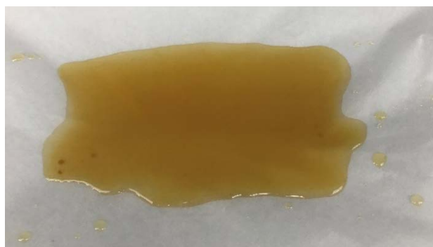
Figure 4. Produced OXE-CHI-PUR polymer.
