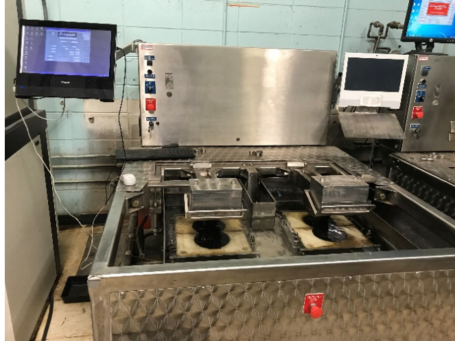
Figure 11. Hamburg loaded wheel tracking test.
