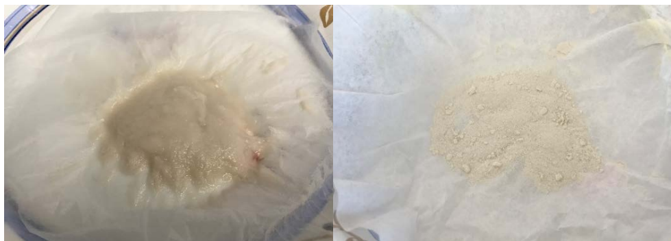
(a) (b) Figure 3. (a) Undried and (b) dried prepared OXE-CHI.
