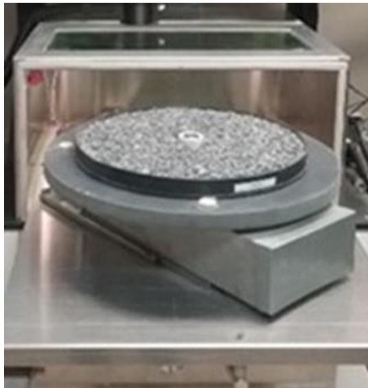
Figure 2.1: SLT Sample Chamber
