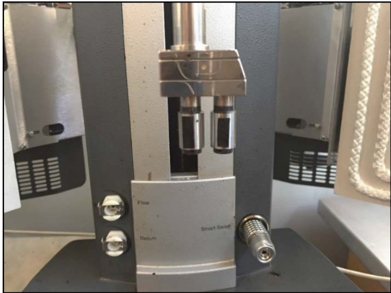
Figure 28. Double-sided adhesive black tape fixed to the drums.
