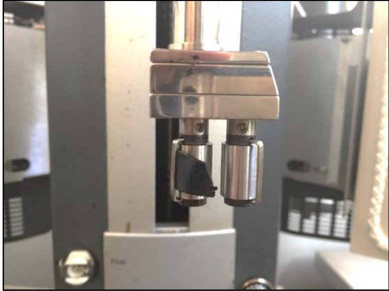
Figure 27. Clamps kicked out due to the hard stresses.
