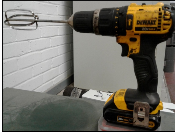
Figure 12. Mechanical mixer used for mixing polymer with asphalt binder.
