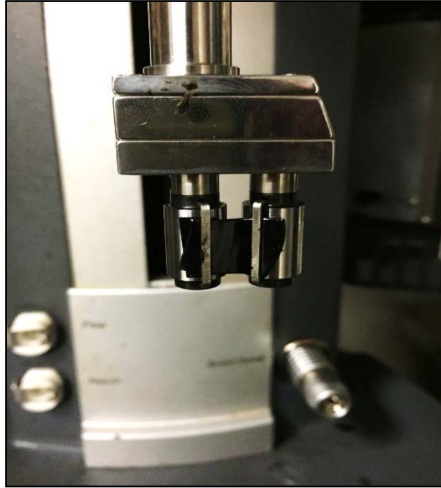
Figure 25. SER fixture after loading the sample.
