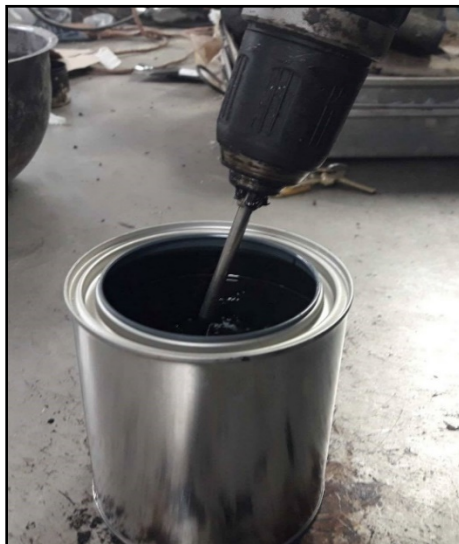
Figure 15. Mixing of polymer with asphalt binder by a mechanical blender.
