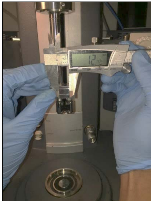
Figure 26. Length of the sample before testing is 12.75 mm.
