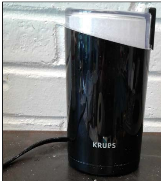
Figure 11. Large size SBS polymer is grinded to smaller size.
