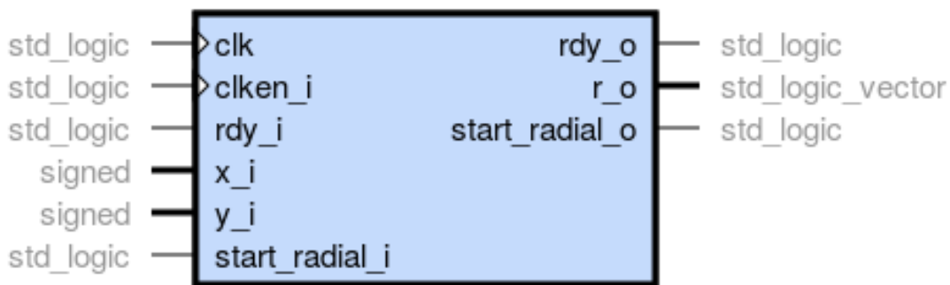
Figure A-17. CORDIC module I/O signals
