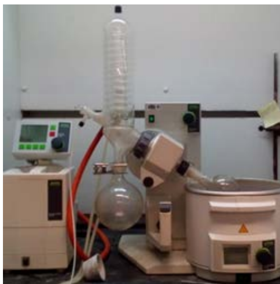
Figure 13. Evaporation of solvents.
