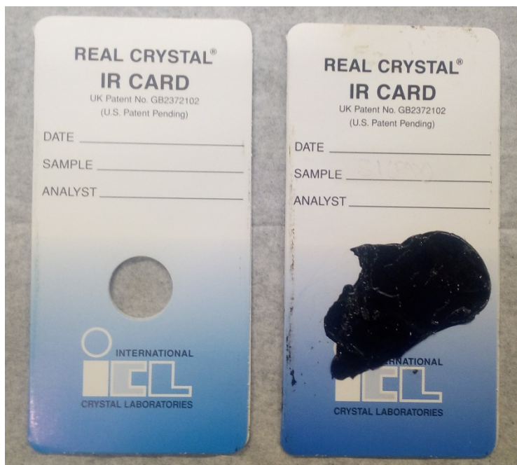
Figure 15. Real crystal IR (KBr) cards.
