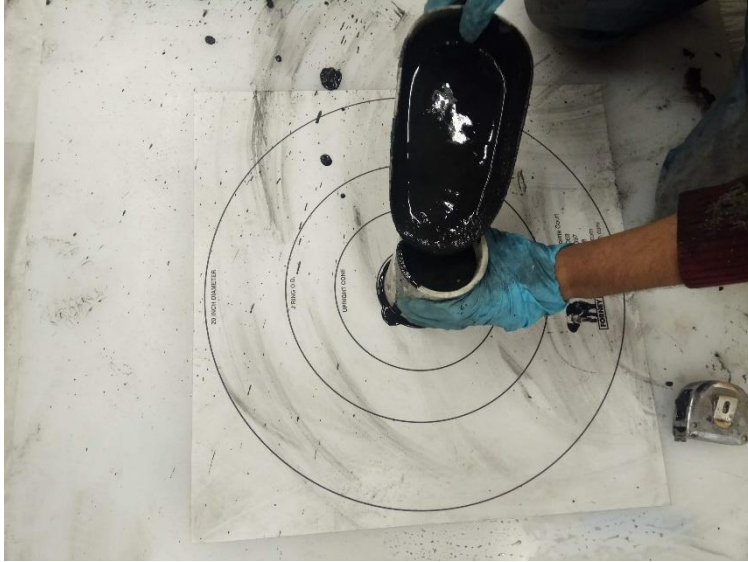
Figure 9. Flow consistency test.
