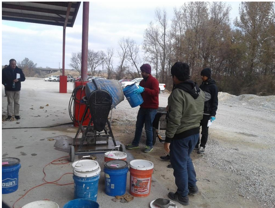
Figure 34. Preparation of an FFC mixture containing 40% 600-RHA and 60% cement.
