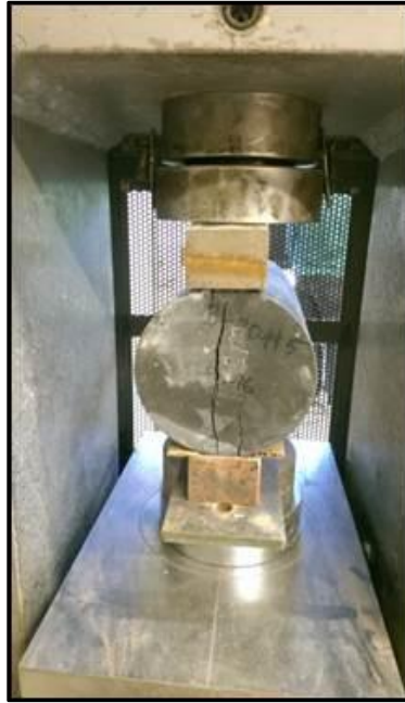
Figure 13. Tensile strength test.
