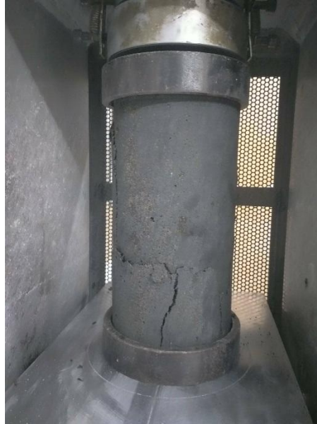
Figure 8. Compressive strength test.
