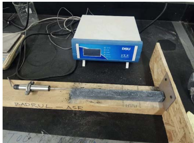
Figure 16. Set up of a linear variable differential transducer (LVDT).
