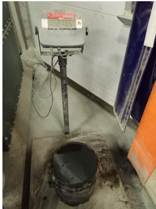
Figure 10. Measuring the unit weight of CLSM mixtures.
