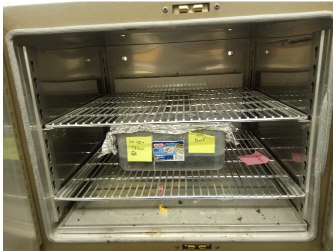
Figure 15. Curing under 1N NaOH solution for the next 14 days.
