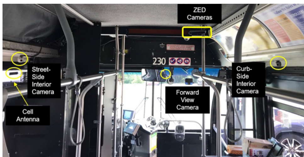
Figure G-2 Instrumentation of NuvoDAS ZED Stereovision, forward, and interior cameras
