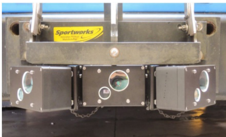
Figure D-2 PASS sensor assembly attached to PT Bus #230
