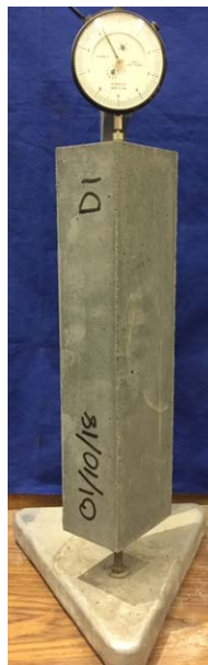
Figure 8. Longer-term shrinkage test setup.
