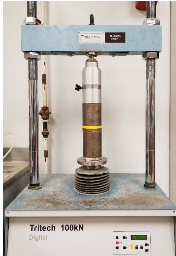
Figure 8. Static compaction of volumetric shrinkage samples.
