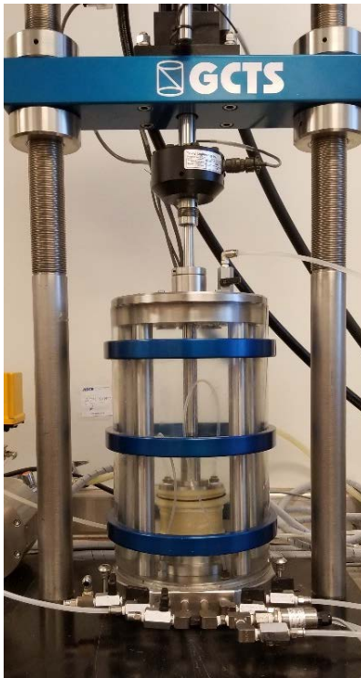
Figure 5. Experimental setup for hydraulic conductivity test.
