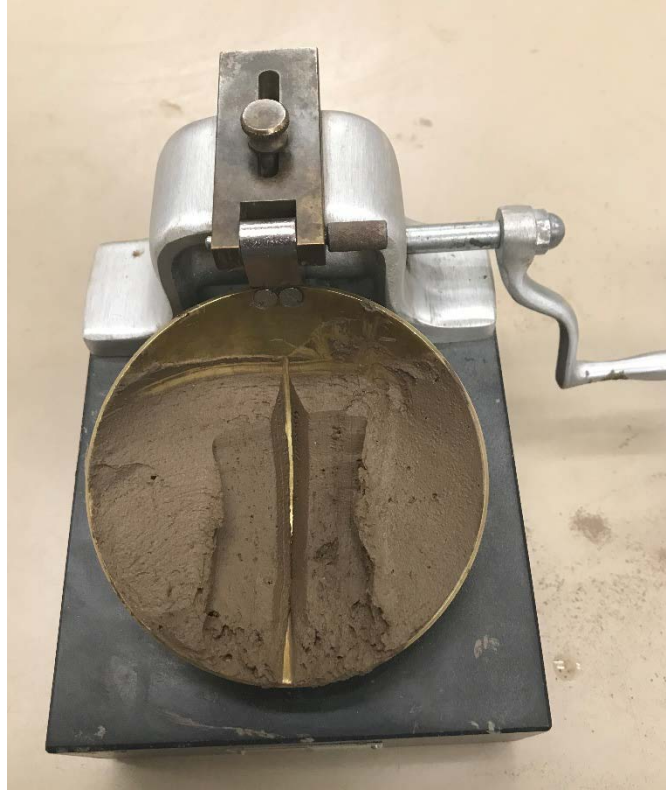
Figure 14. Liquid limit test of the soil sample in Casagrande device.
