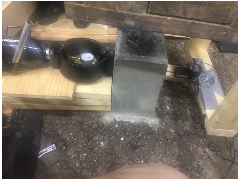
Figure 33. Inclination of drilled shaft.
