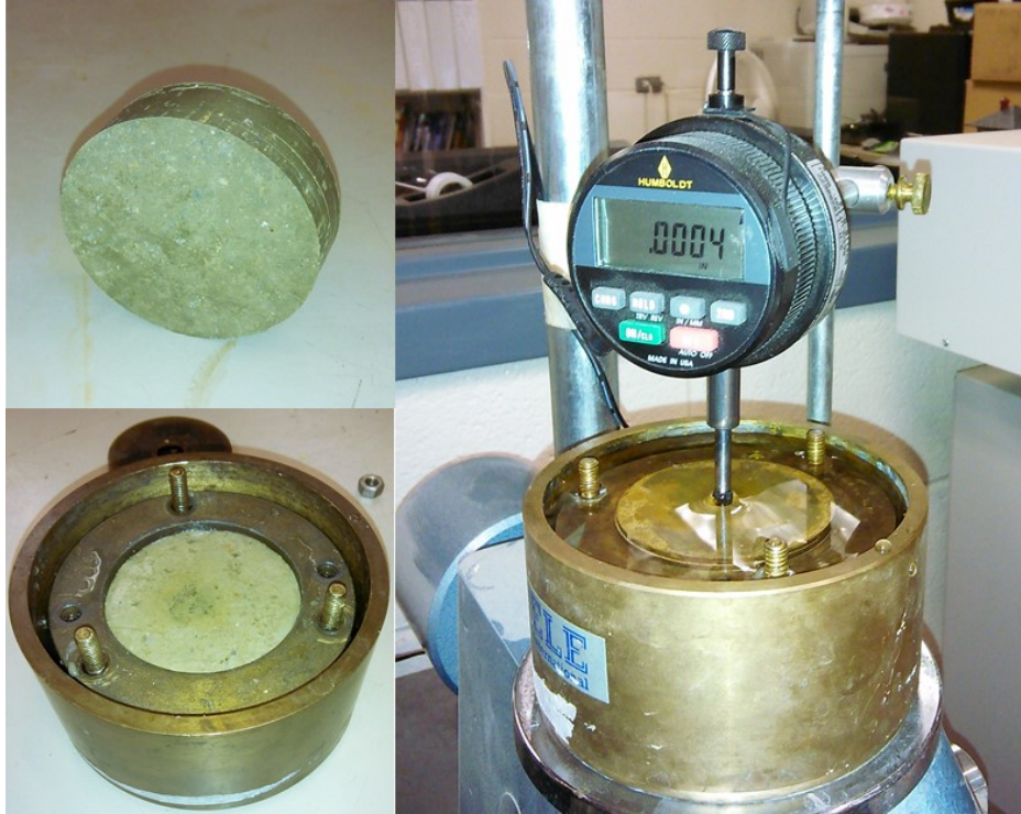
Figure 19. One-dimensional consolidation test: (top-left) soil sample in brass ring, (bottom-left) setup of fixed ring consolidometer, and (right) dial-gauge reading during the test.
