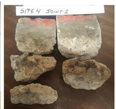
Figure 15. Cores from buckling sites taken from transverse joints and core holes showing spalls in the lower portion of the joint.
