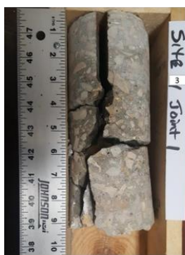
Figure 15. Cores from buckling sites taken from transverse joints and core holes showing spalls in the lower portion of the joint.
