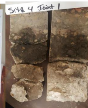
Figure 15. Cores from buckling sites taken from transverse joints and core holes showing spalls in the lower portion of the joint.
