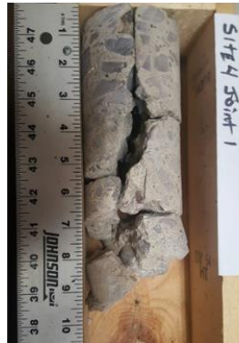
Figure 15. Cores from buckling sites taken from transverse joints and core holes showing spalls in the lower portion of the joint.
