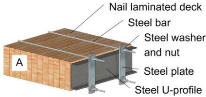
a) Measure of repair of nail-laminated decks;
