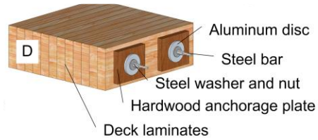
d) Prestressing system normally used in Sweden
