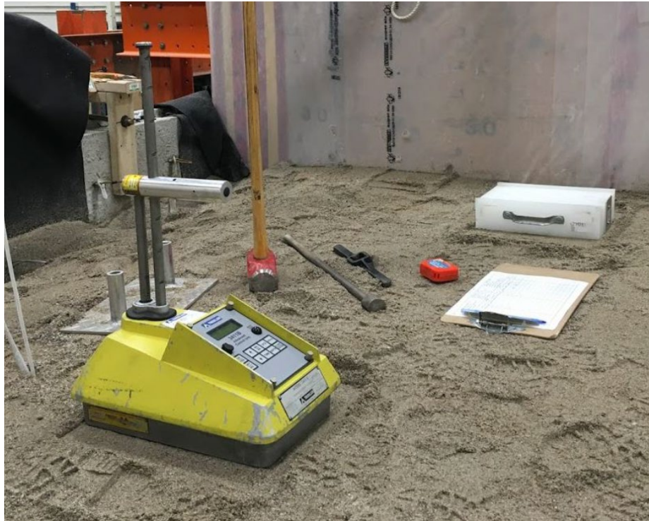
Figure 3-8. Nuclear densometer – Troxler 3411_B.
