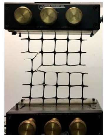
A biaxial geogrid ruptures during ASTM D6637 Method B testing.
