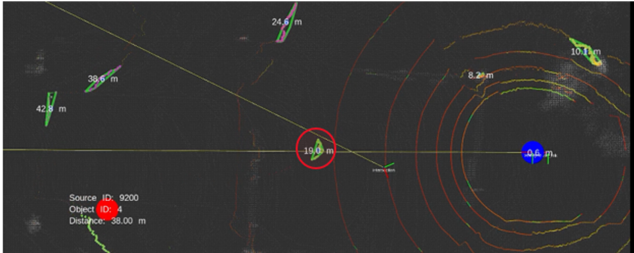
Figure 5-27: Simultaneous detection of the conventional vehicle by the intersection and CAV.
