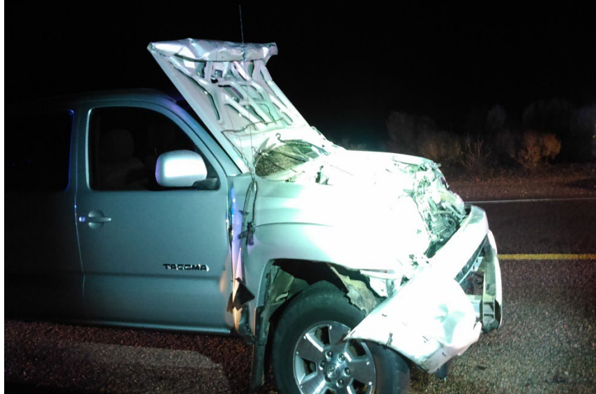
Figure 2. Vehicle Damage Caused by a BVC
