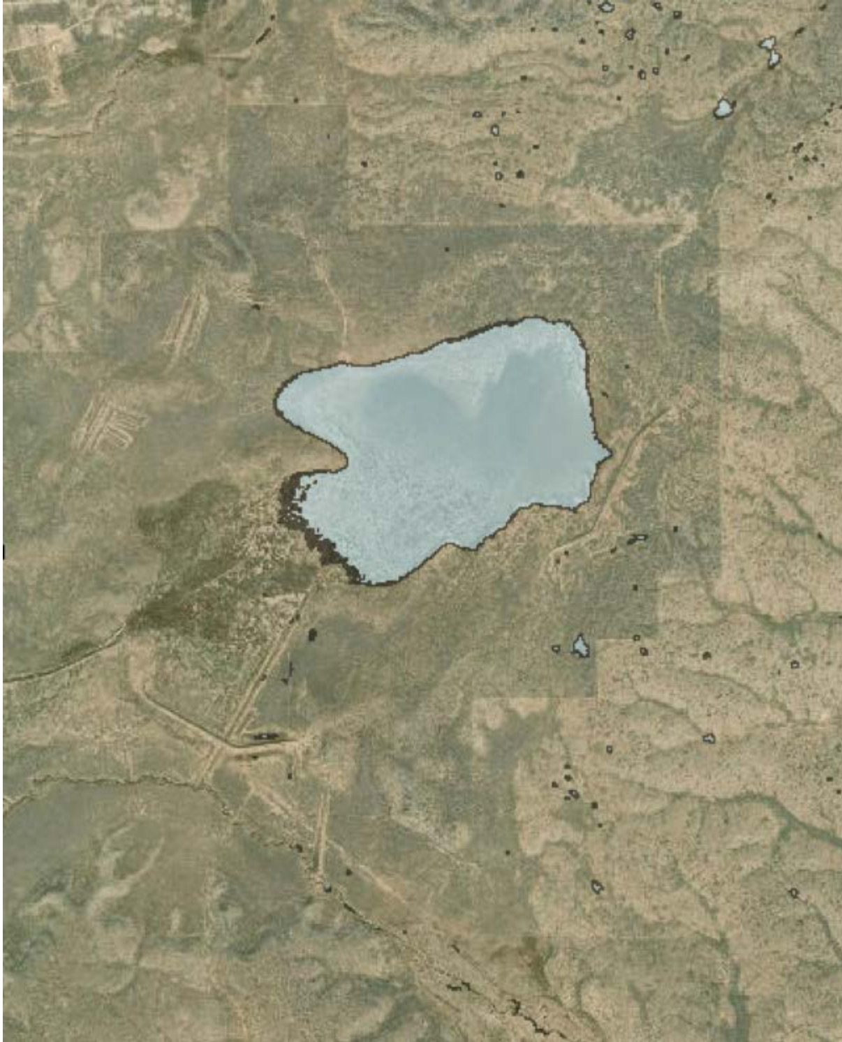
Figure 25. A false positively detected sinkhole which is actually a reservoir.
