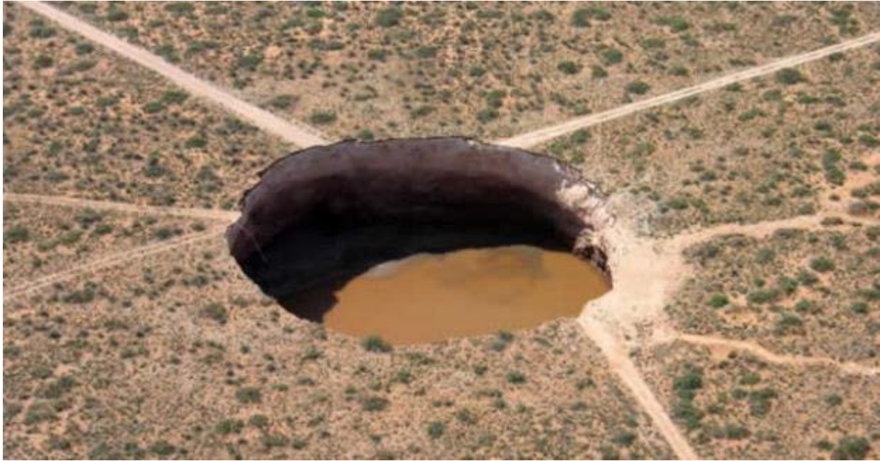
Figure 8. Sinkhole detection principle of identifying the distinct shape-transition boundary in reference to the surrounding terrain (adopted from NCKRI).
