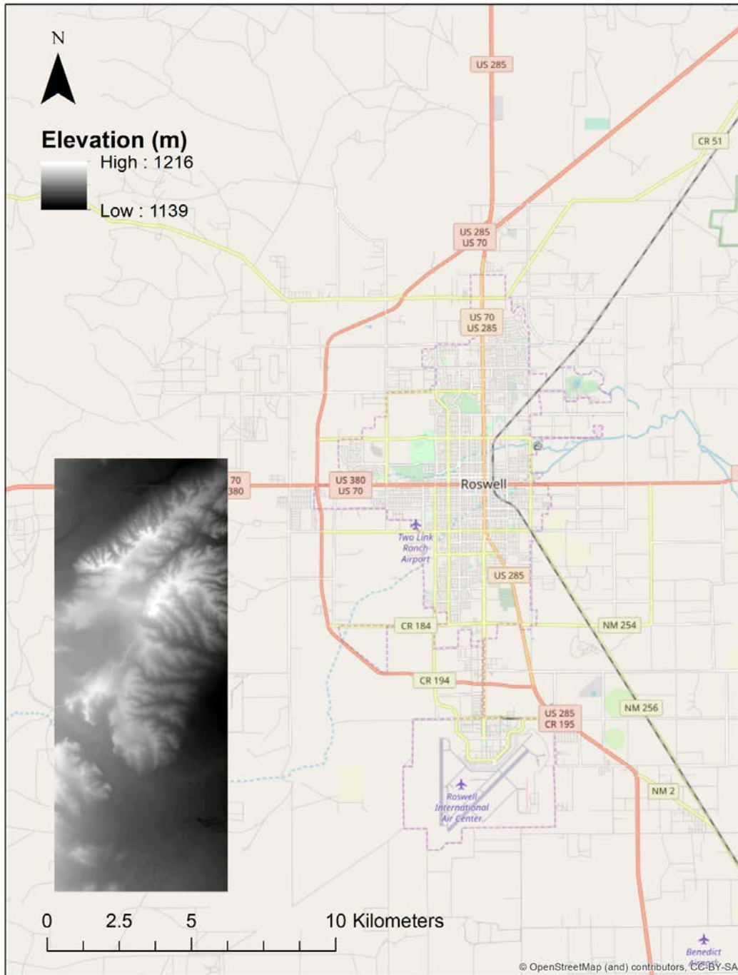
Figure 19. The mosaicked DEM layer when using multiple LAS tiles as input.
