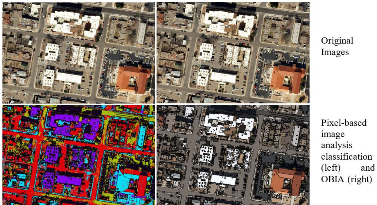
Figure 14. Pixel-based image analysis classification vs. OBIA classification.
