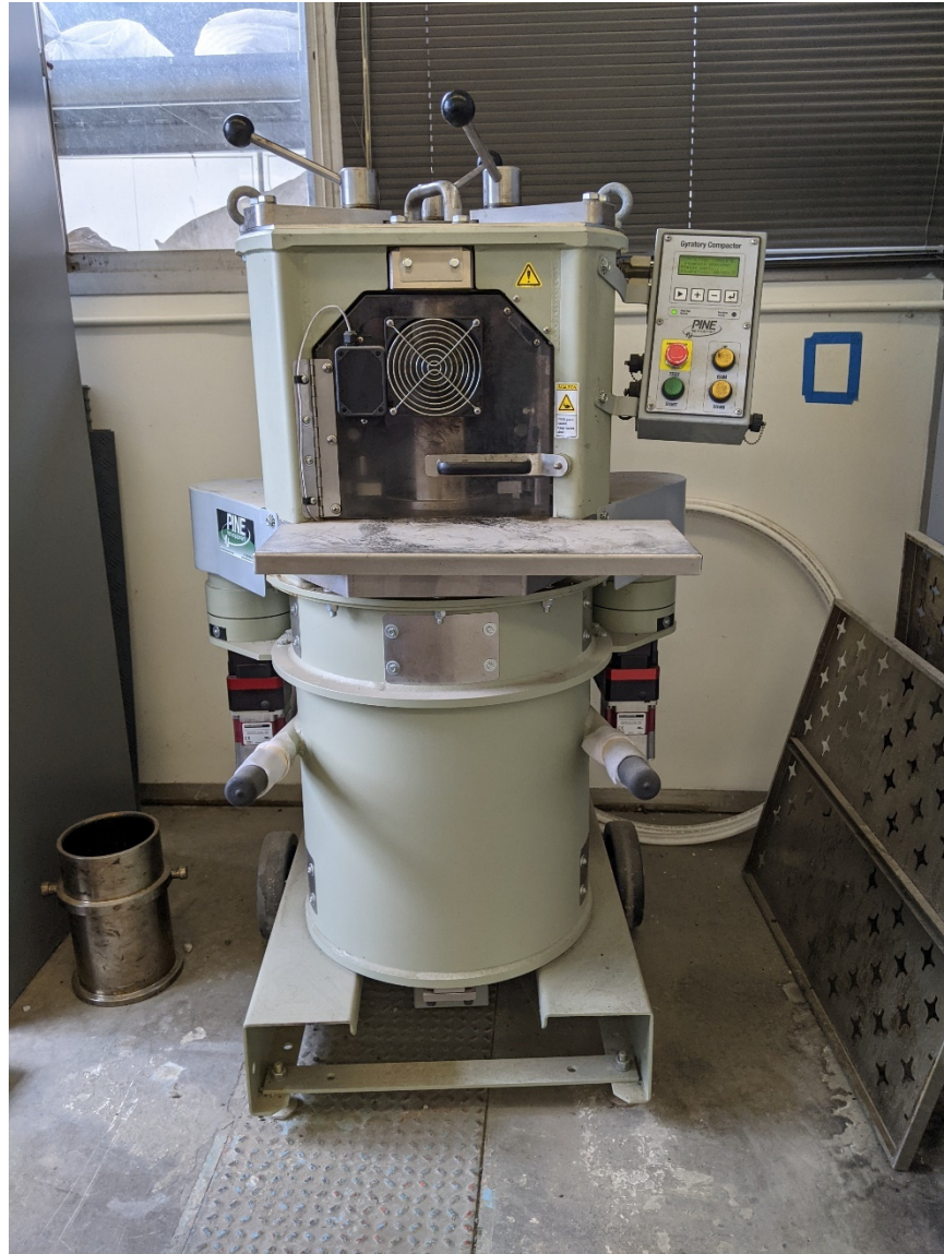
Figure 4. (b) Pine Superpave Gyratory Compactor Compacting the G5 Sample
