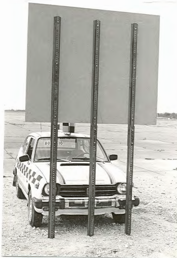
FIGURE A-78. RELATIVE POSITIONS OF TEST VEHICLE AND SIGN INSTALLATION FOR TEST 10.
