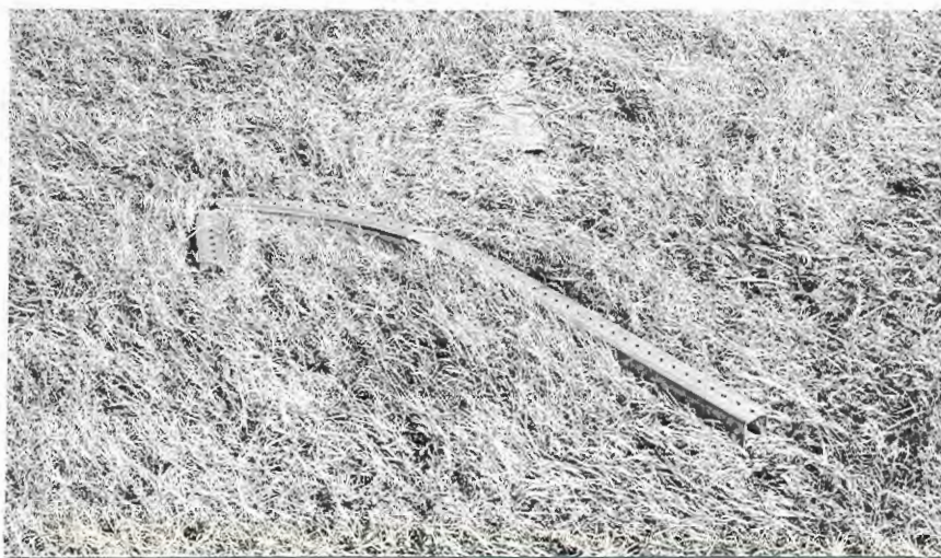
FIGURE A-56. SIGN INSTALLATION AFTER TEST 6. (SUPPORTS AND SIGN PANEL)
