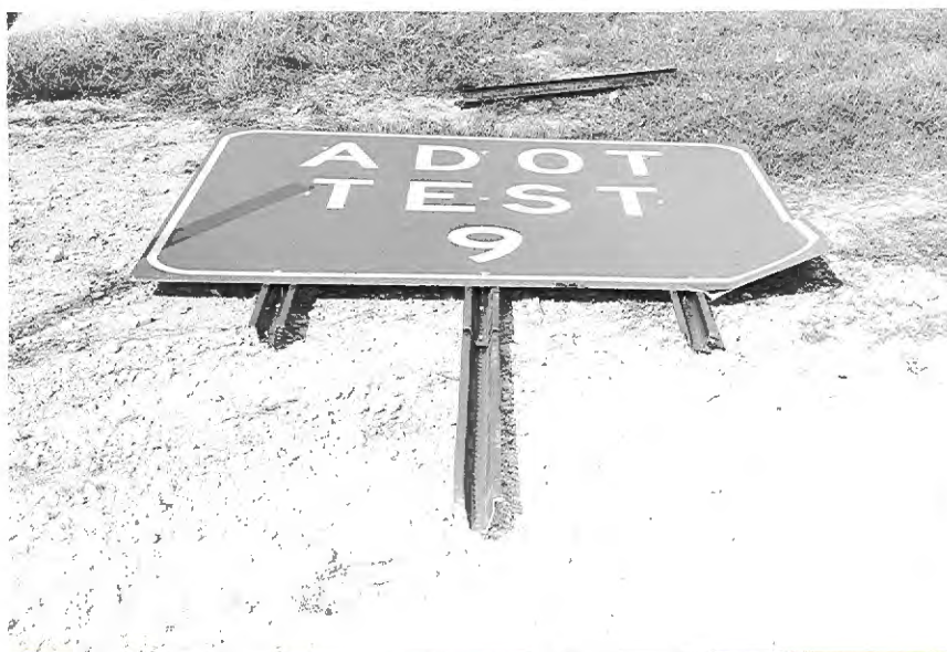
FIGURE A-74. SIGN INSTALLATION AFTER TEST 9.
