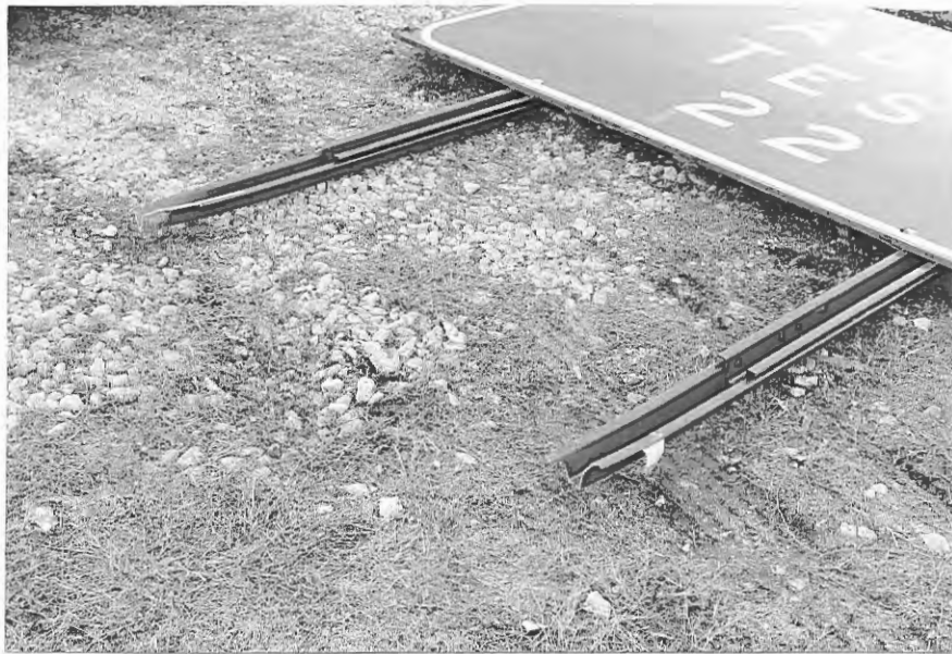
FIGURE A-142. SIGN INSTALLATION AFTER TEST 22.
