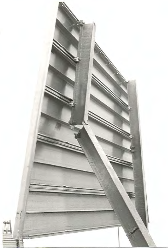
FIGURE A-24. SIGN INSTALLATION AFTER TEST 1.
