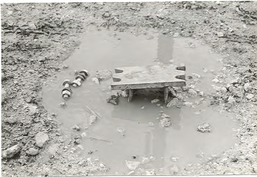
FIGURE A-25. BREAKAWAY BASE AFTER TEST 1.
