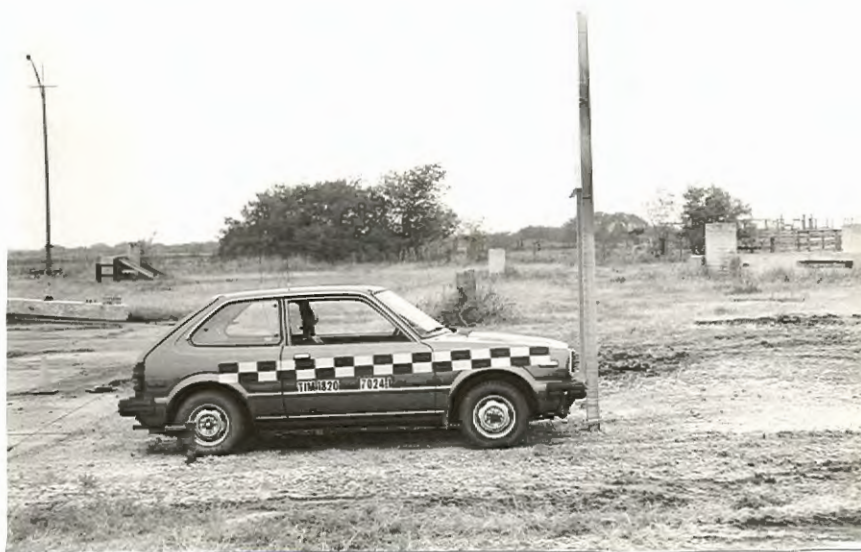
FIGURE A-23. RELATIVE POSITIONS OF SIGN INSTALLATION AND TEST VEHICLE FOR TEST 1.
