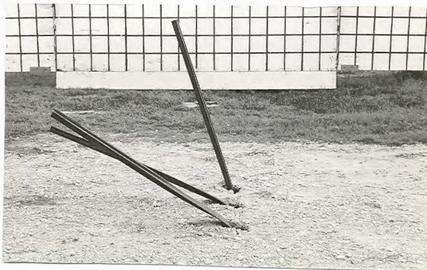
FIGURE A-79. SIGN INSTALLATION AFTER TEST 10.
