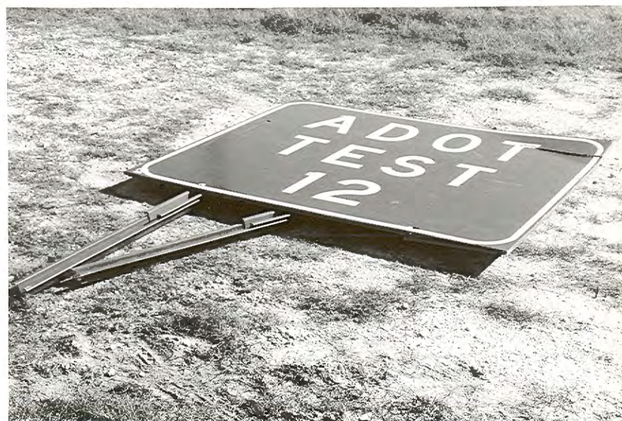
FIGURE A-90. SIGN INSTALLATION AFTER TEST 12.
