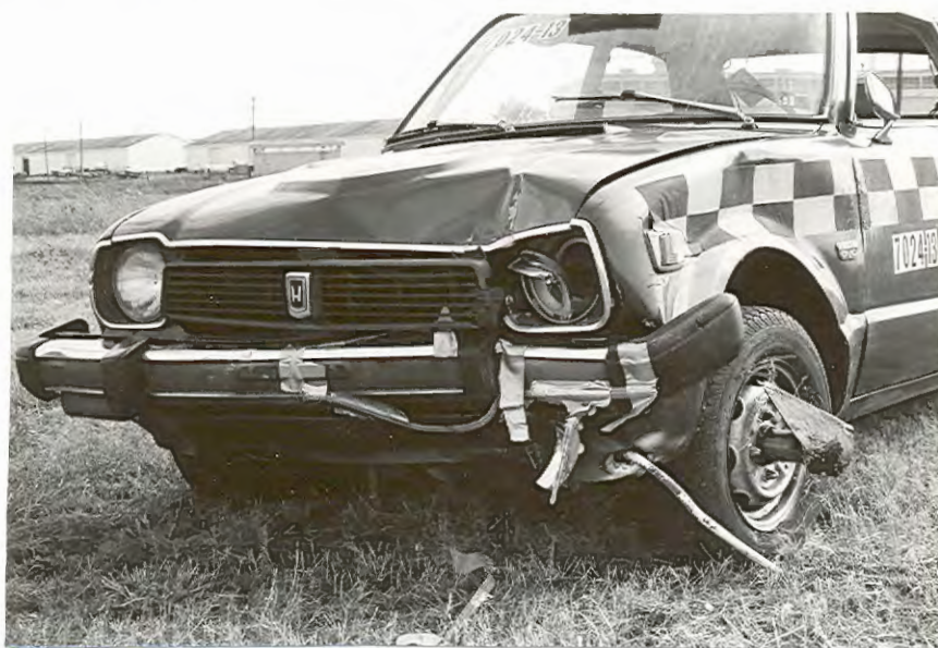
Post-test roll attributed to unsymmetrical brake application and soil condition.
