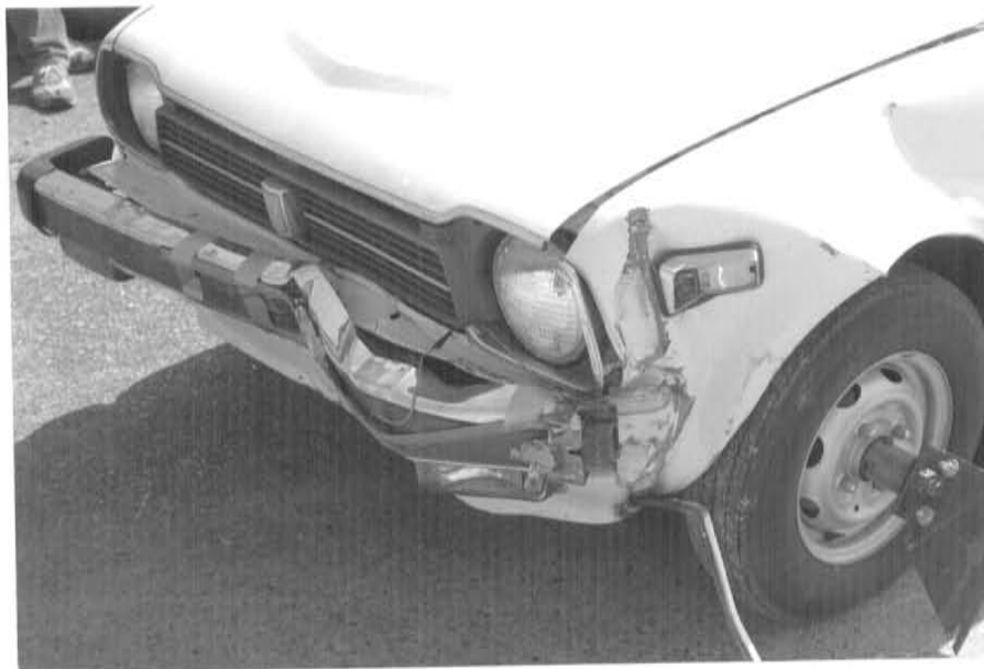
FIGURE 7.5. VEHICLE DAMAGE FOLLOWING TEST 7024-24.
