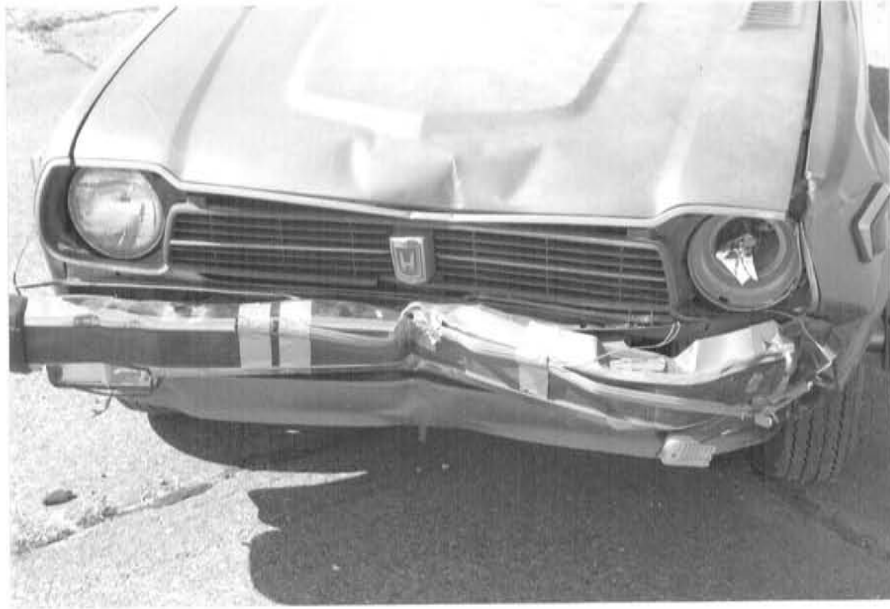
FIGURE 7.21. VEHICLE DAMAGE FOLLOWING TEST 7024-27.
