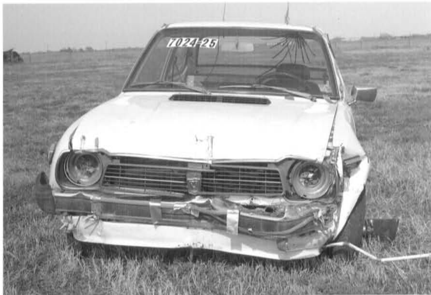
FIGURE 7.10. VEHICLE DAMAGE FOLLOWING TEST 7024-25.
