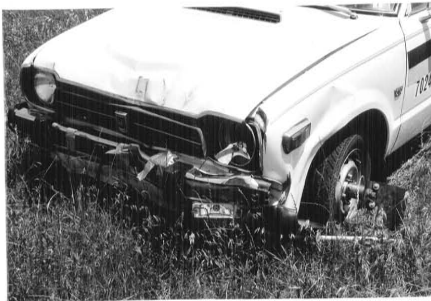
FIGURE 7.32. VEHICLE DAMAGE FOLLOWING TEST 7024-30.
