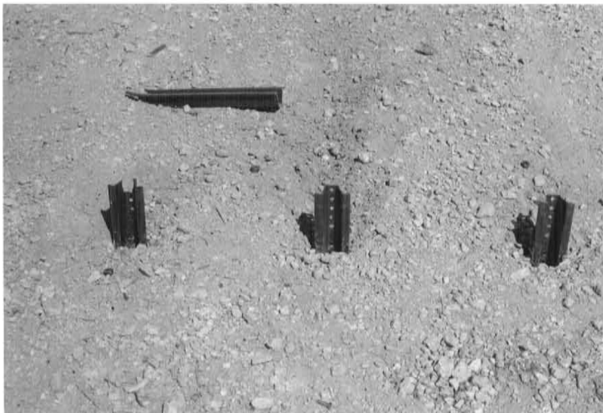
FIGURE 7.15. SIGN SUPPORTS FOLLOWING TEST 7024-24.
