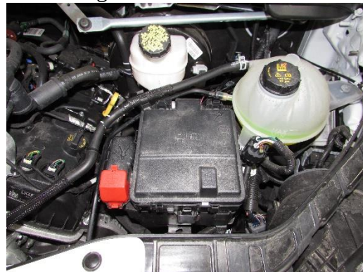
Battery cable terminal in engine compartment
