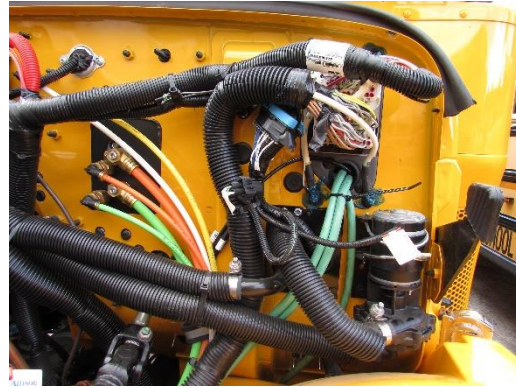
Firewall on right side
