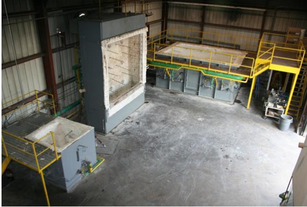
Figure 1. SwRI's fire resistance furnaces
