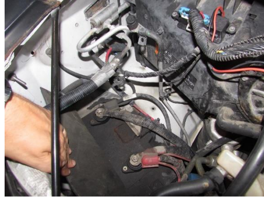
Showing battery under/adjacent HVAC
