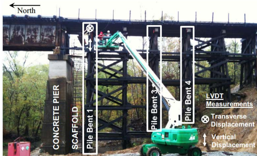
Figure 2. Measuring railroad bridge displacements in the field (14, 15).
