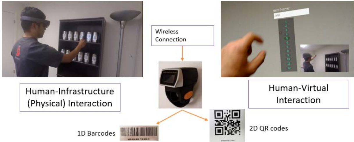
Figure 21. AR headset (Microsoft HoloLens) was used to build a system architecture where inspectors could go to site, connect to the remote server and quickly view information by scanning unique barcode.
