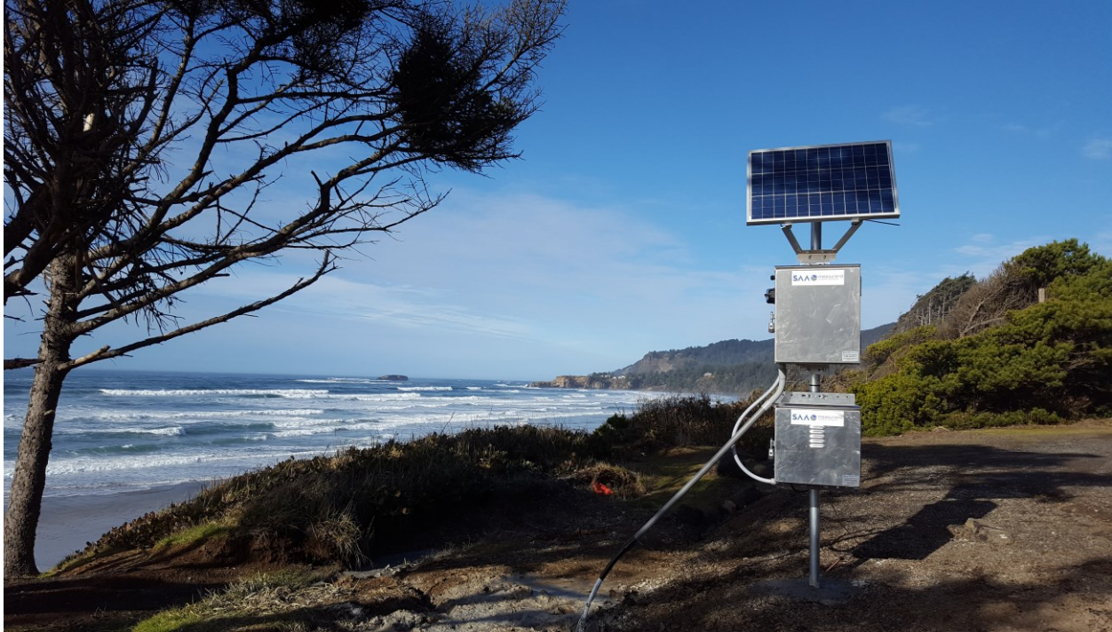
Figure 2.13: Final SAA MEM’s sensor setup at Spencer Creek on January 27, 2017. Composed of solar panel for power supply, SAA electrical components (top box), SAA battery (bottom box), and SAA sensor (in borehole). Photograph Credit: Dr Michael Bunn.
