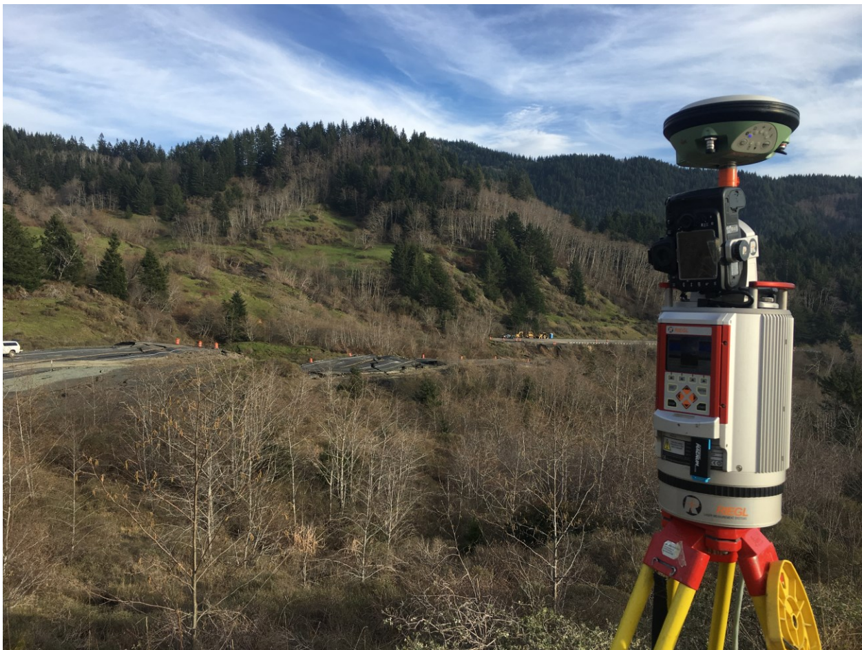
Figure 2.7: Photograph of Riegl VZ-400 TLS setup to conduct high resolution repeat scans of the actively moving Hooskanaden landslide on March 2, 2019.
