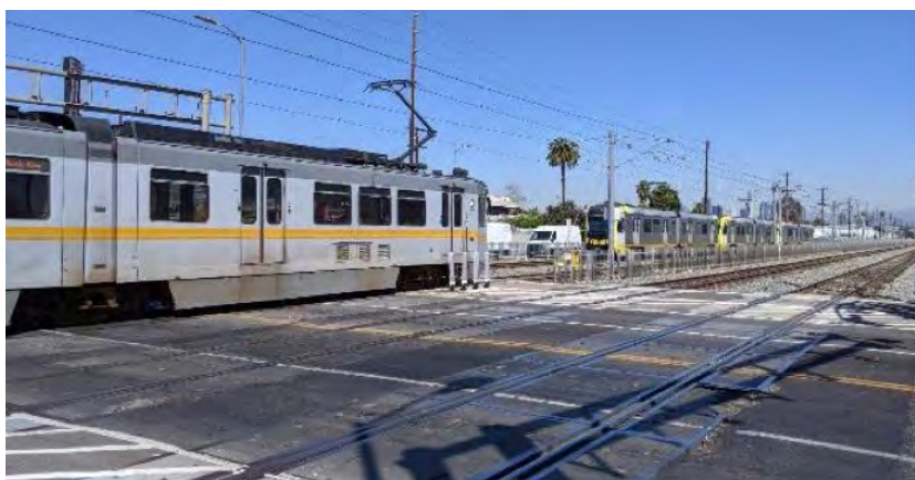
Figure 6-21 Two trains at grade crossing on different tracks at nearly same time
