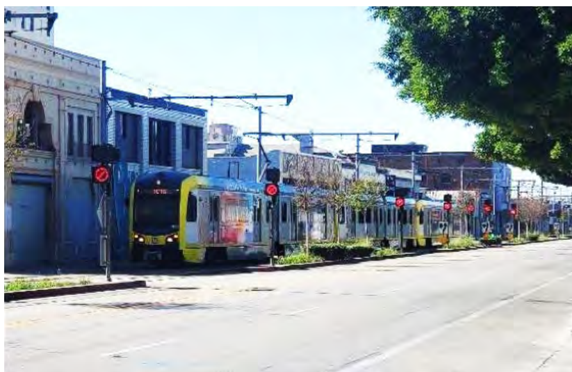
Figure 6-25 Dynamic signs prohibiting left turns into driveways in presence of train; train presence sign dark – second in sequence
