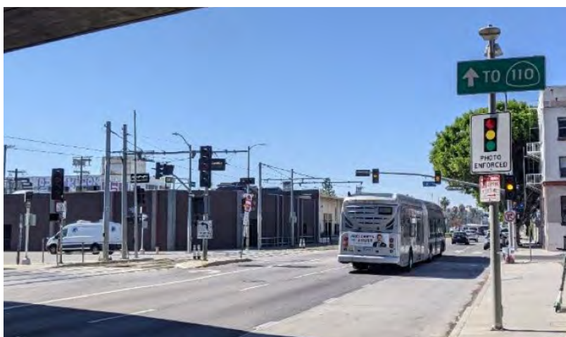
Figure 6-29 Traffic sign indicating photo enforcement at street-running grade crossing intersection
