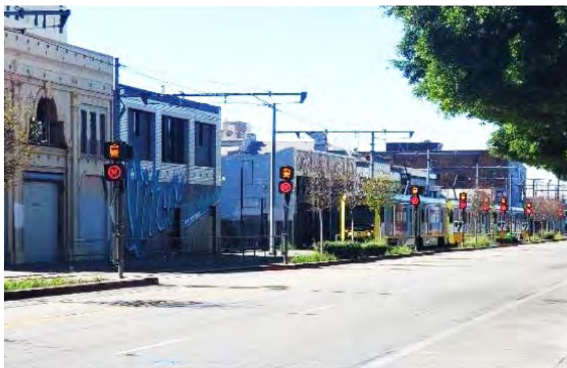
Figure 6-24 Dynamic signs prohibiting left turns into driveways in presence of train; train presence sign illuminated – first in sequence
