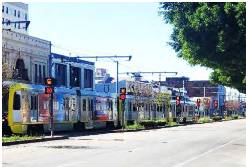
Figure 6-26 Dynamic signs prohibiting left turns into driveways in presence of train; train presence sign flashing – third in sequence
