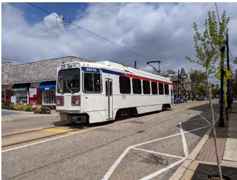
Figure 6-105 Double-ended car with pantograph on single track street-running at end of Route 101 in Media
