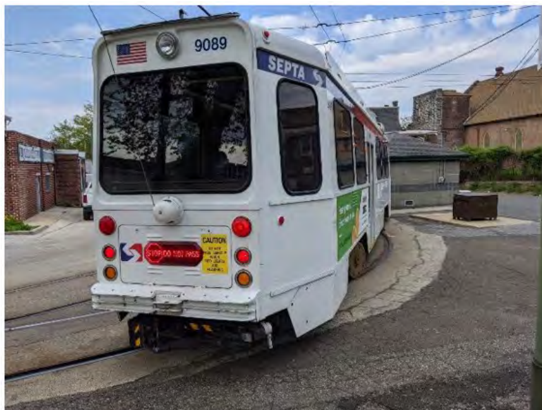
Figure 6-99 Special brake-activated message and signage to reduce rear-end collisions on city trolleys
