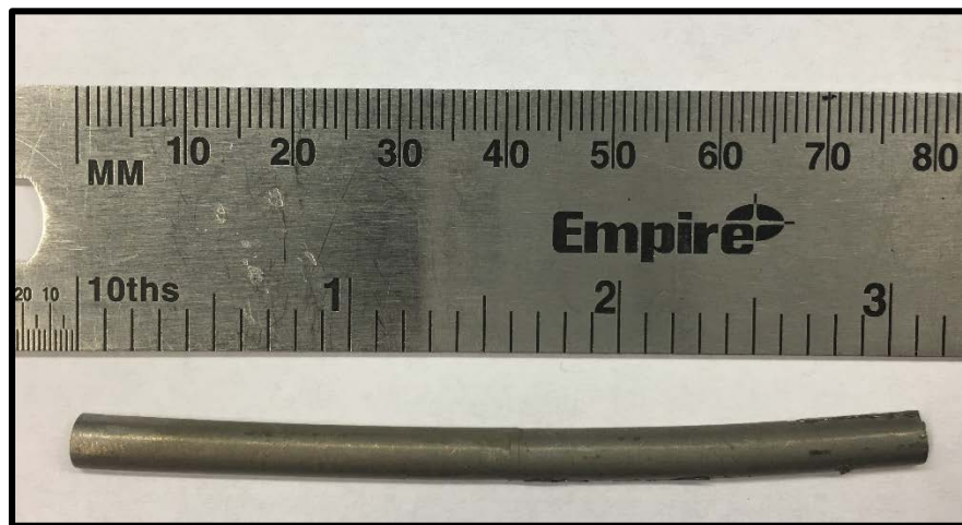
Figure 7. FeMnAlNi bar with 4.6 mm diameter subjected to abnormal grain growth heat treatment between 1200°C and room temperature.
