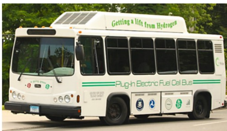
Figure 3-18 GNHTD fuel cell plug-in hybrid-electric transit bus manufactured by Ebus
