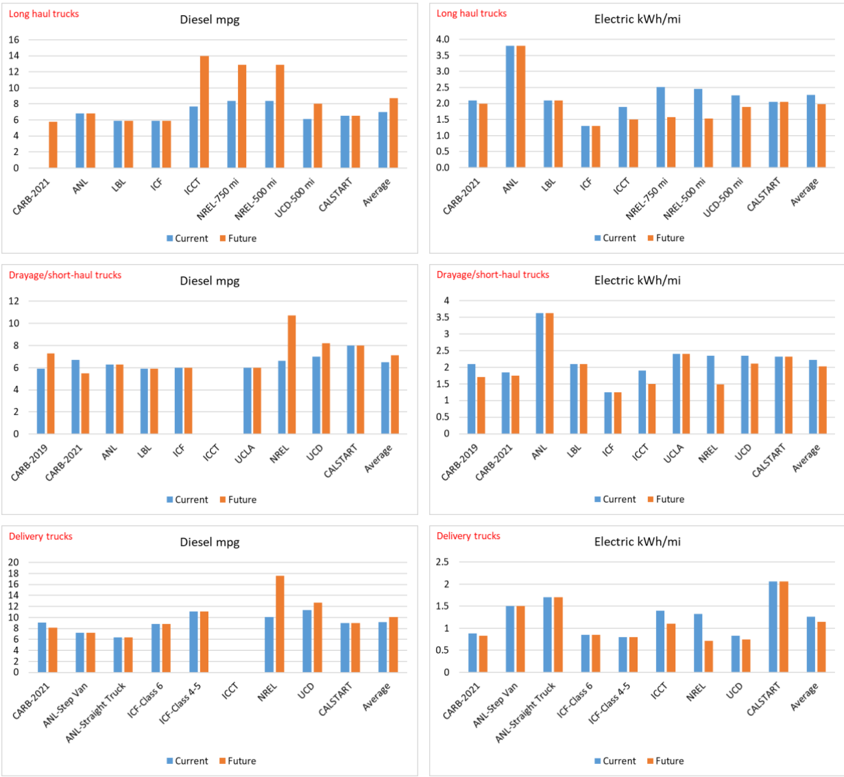
Figure 17. Fuel economy or energy consumption rates comparison across studies and truck types (MPG for diesel and kWh/mi for electric)
